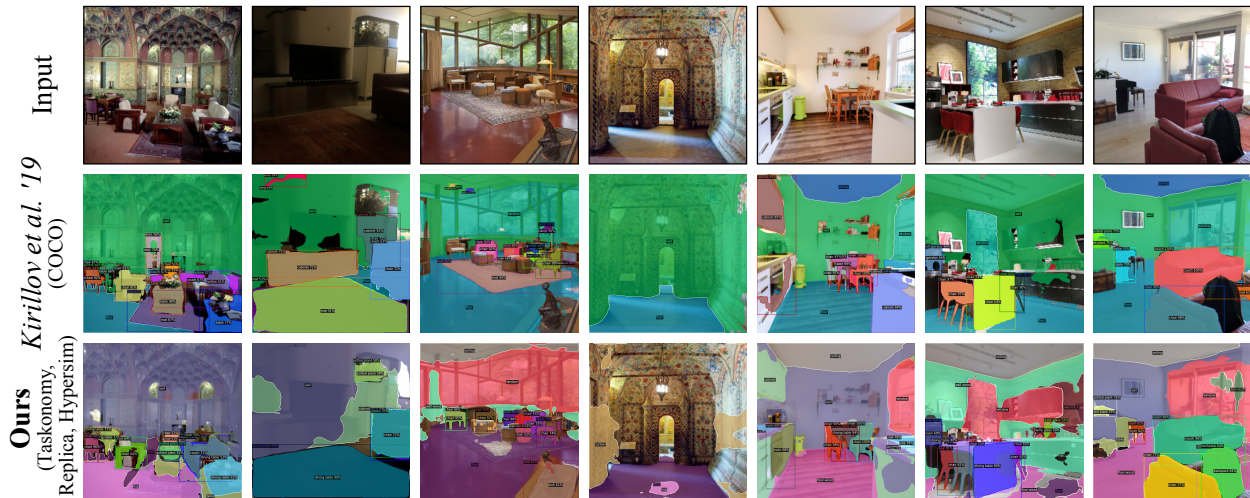
Figure 5.7: Qualitative results of panoptic segmentation with PanopticFPNs [110] trained on COCO [130] and Omnidata . The Omnidata model trained jointly on Taskonomy, Replica, and Hypersim shows good out-of-distribution performance on indoor scenes without people.
