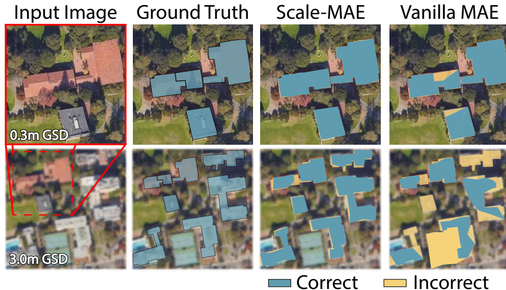
Figure 5.1: Scale-MAE learns better representations for multiscale tasks compared to vanilla MAE. (Column 1) The top image spans an area at 0.3m GSD and the bottom image shows the same region at a coarser GSD. (Columns 2-4) The following columns show a ground truth building segmentation, Scale-MAE segmentation from a finetuned UperNet, and segmentation from an analogously finetuned UperNet from a vanilla MAE, respectively. Scale-MAE demonstrates better performance across images at both scales. See the supplementary material for more examples.
