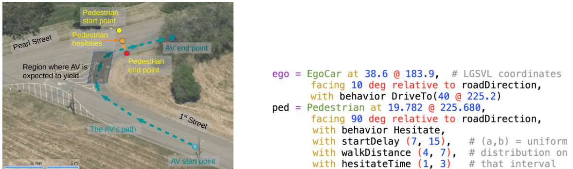
Figure 5.3: A bird's-eye view of the scenario S (left) and the (simplified) SCENIC program P_S encoding our test scenario.
