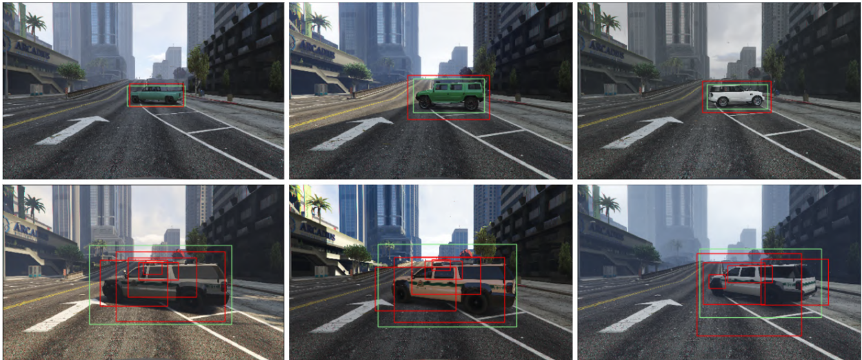
Figure 4.5: The top (or bottom) three images are generated using the refined SCENIC program with the correct (or incorrect) detection inducing rule shown in Table 4.2 (or Table 4.4) for Scenario 1. The green boxes are the ground truth bounding boxes for the detection task, and red boxes are the predictions of the pre-trained perception model used in this study.
