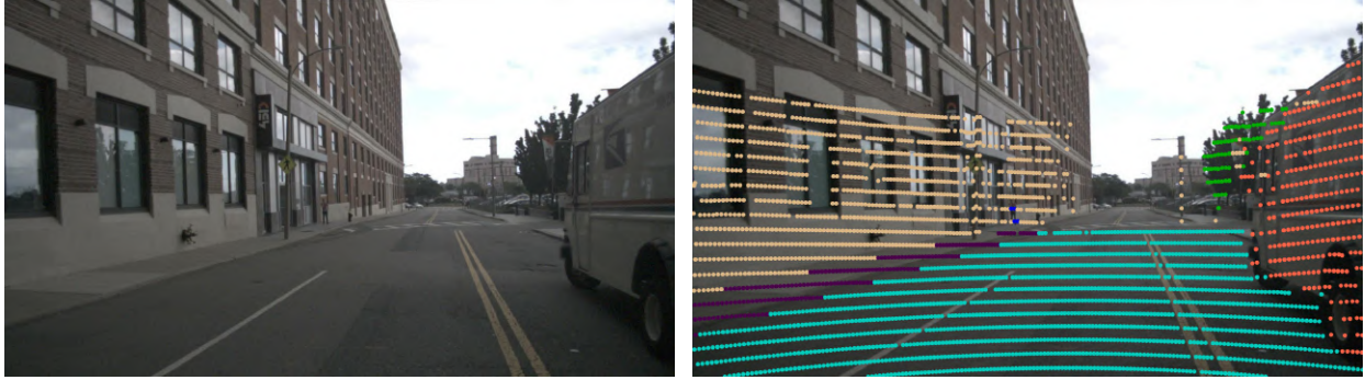
Figure 6.2: A benefit of querying a label is that we can retrieve corresponding sensor data of multiple types. Here, our algorithm finds both an RGB image and a segmented 3D LiDAR point cloud corresponding to a single label.
