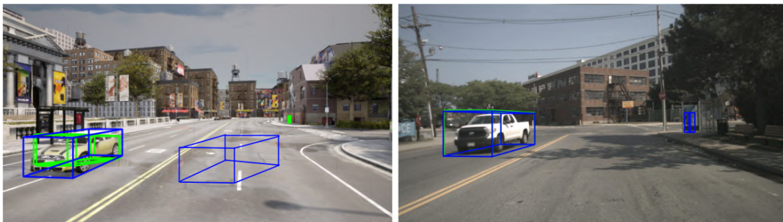
Figure 5.1: The discrepancy in the behaviors of a neural network-based perception model on the synthetic (left) versus the real (right) RGB camera images are shown. The contents of the two images are similar, where a single vehicle approaches from the opposite traffic. However, the perception on the synthetic image results in a false detection of a non-existent vehicle. The green boxes represent the ground truths, and the blue represent detections by the neural network.
