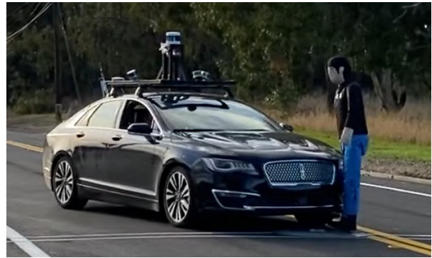
Figure 5.5: The autonomous vehicle and pedestrian dummy used for track testing. The picture shows the AV hitting the pedestrian during testing (test F1 Run 1, https://youtu.be/PehgLCGHF5U ), see Section 5.3.1 for details.
