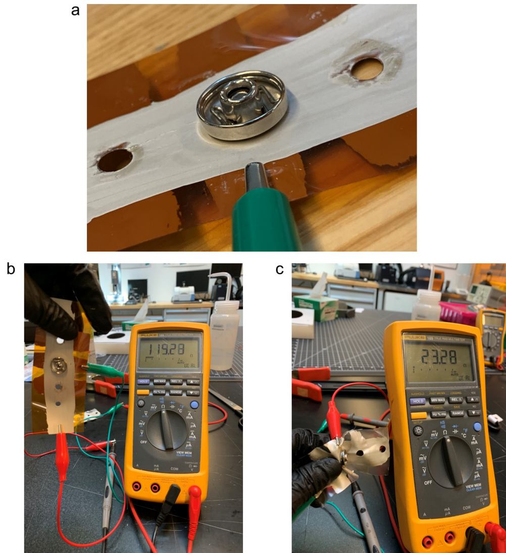
Figure 6.2: Prototype screen-printed via with eyelet reinforcement. (a) Screen-printed traces on flexible Kapton substrate with eyelet reinforcement. (b) and (c) Resistance measurement of unflexed via on Kapton and flexed via on Dupont Intexar substrates, respectively.
