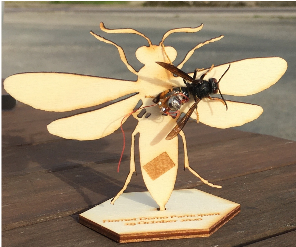
Figure 3.11: Tracker attached to Hornet [94]
