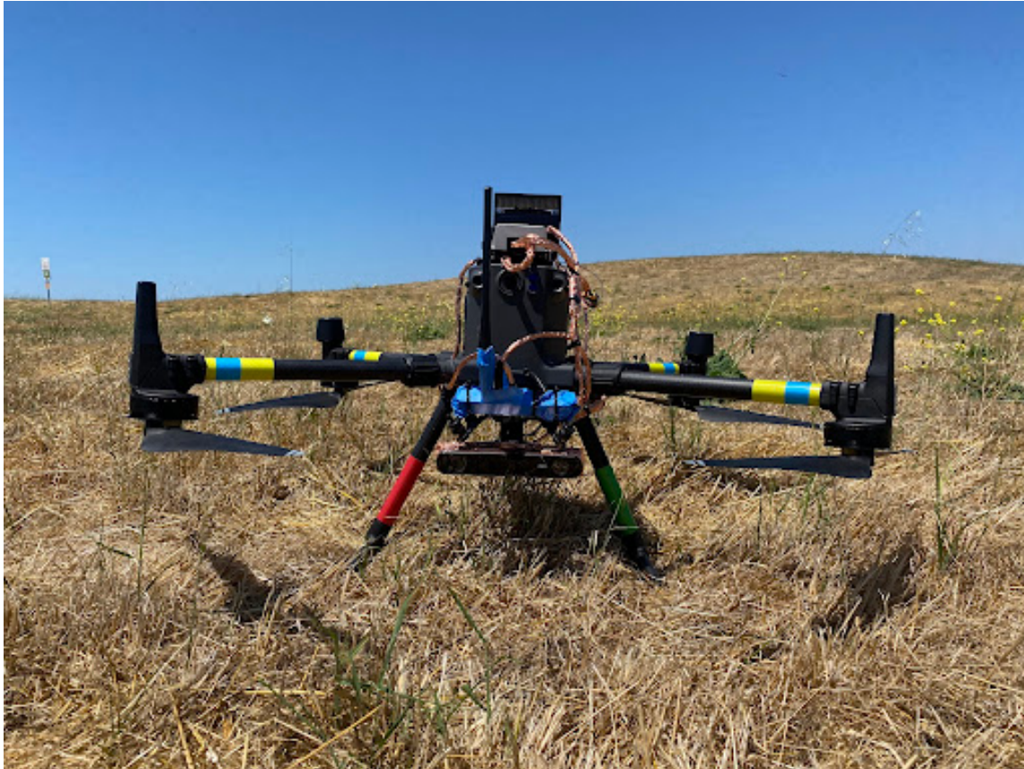
Figure 2.10: The physical platform, including a DJI Matrice 300 drone, ZED2i camera, and Jetson Xavier AGX.
