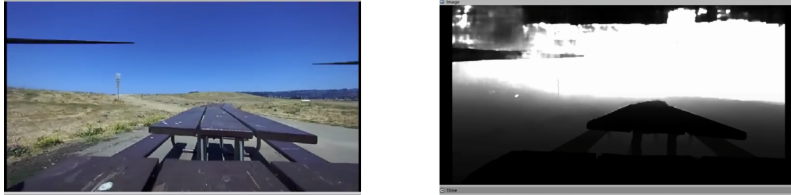
Figure 2.11: Propellers block the camera’s field of view, resulting in noisy depth images. Left, an RGB image from the camera showing propellers jutting out from both sides of the image. Right, the depth image showing noise values where the propellers are rapidly spinning. This section is masked out before being passed to the policy.
