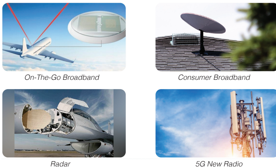
Figure 1.1: Examples of applications using phased arrays.
