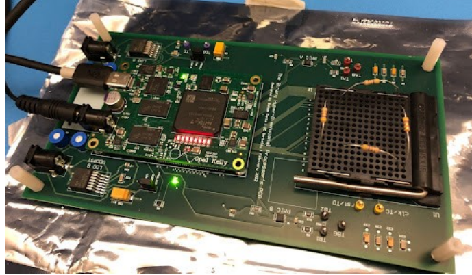
Figure 6-4: Calibrating the sense-resistor for VDD current measurements. Load resistors 5.3, 5.3, 5.3 and 5.2 Ohms were connected in parallel between core voltage supply VDD and common ground GND. The PMIC shunt voltage read 176716 which indicates 55.2 mV. The load resistors draw about 0.758 A from the VDD supply rail, indicating the sense resistor's value is about 0.0728 Ohm.
