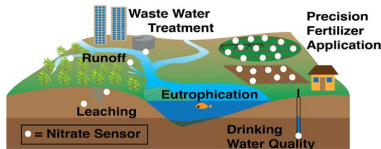
Figure 1.6: Nitrate enters an ecosystem through fertilizer application in agricultural settings or from wastewater. From there, it leaches to groundwater, contaminating wells used for drinking water, or runs downstream to cause eutrophication in surface waters. Improved monitoring through a distributed sensor network could help map the movement of nitrate through the landscape.
