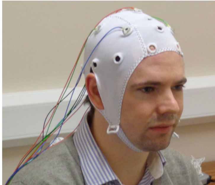
Figure 1.2: Lab based electroencephalogram used for measuring neural activity from the scalp with metal electrodes. Reproduced from [26] with permission.
