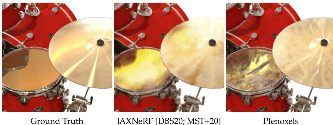
Figure 2.9: Artifacts. JAXNeRF and Plenoxel exhibit slightly different artifacts, as shown here in the specularities in the synthetic drums scene. Note that some artifacts are unavoidable for any underdetermined inverse problem, but the specific artifacts vary depending on the priors induced by the model and regularizer.
