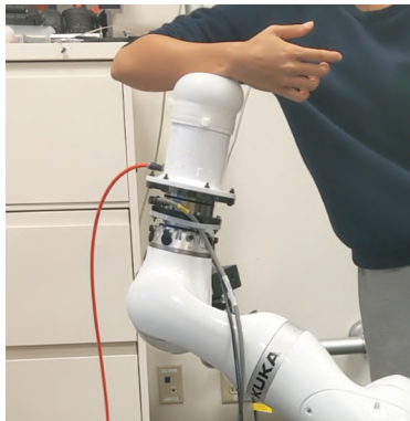
Figure 3.1: The proposed soft interface enables safe and precise tactile interaction between a human and a robot. ©2020 IEEE.
