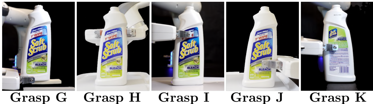
Figure 6.12: Five tested grasps on a real bleach bottle. Grasps are also repeated in simulation. ©2022 IEEE.
