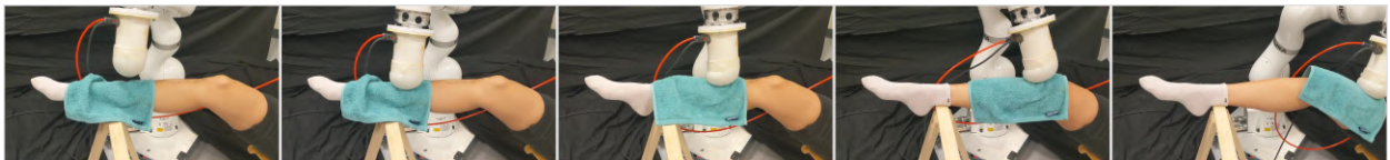
Figure 4.9: The robot cleans the the length of a leg with a damp washcloth and maintains constant contact even over the knee. ©2022 IEEE.
