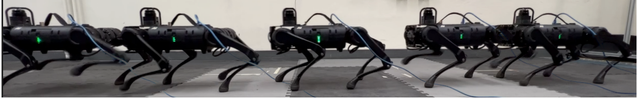
Figure 2.1: We learn precise tracking policy on hardware for the Unitree A1 Quadrupedal robot [85] using less than 20 seconds of data. A video of our experiments can be found here https://youtu.be/l7kBfitE5n8
