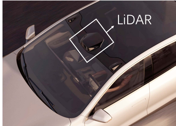
Figure 2.1: LiDAR module on a car with advanced driving assistance function.
