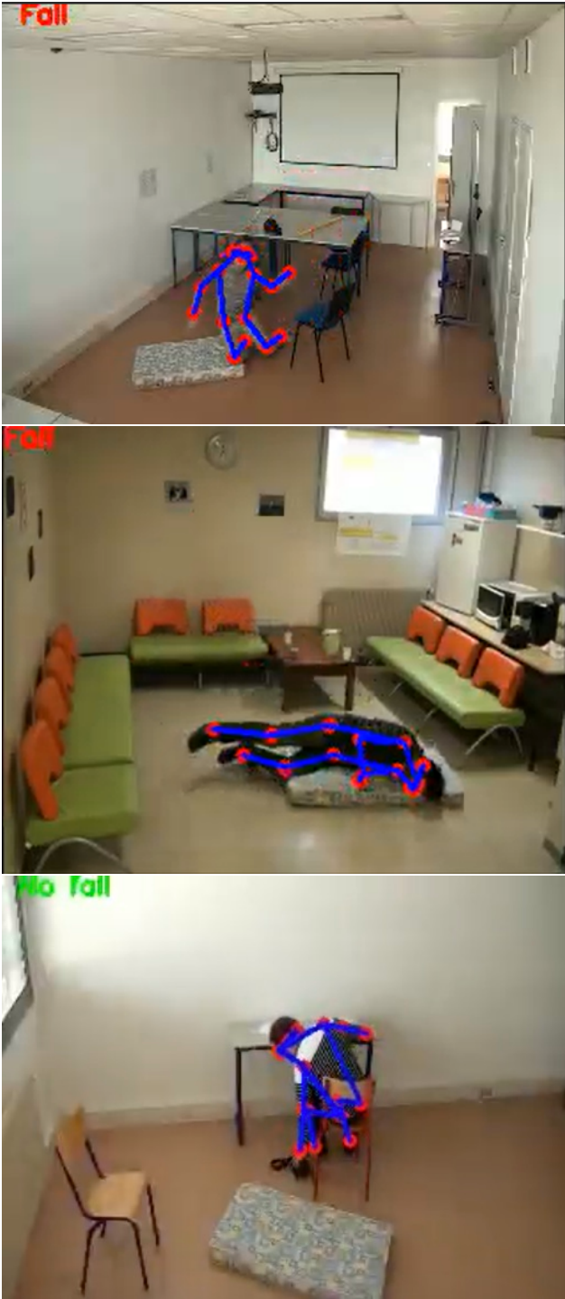
Figure 5.4: Demonstration of the proposed fall detection method. Top: detect "Fall" in the test video. Mid: detect "Fall" in validation video. Bottom: detect "Non-Fall" in the test video. Full videos: top , mid , bottom
