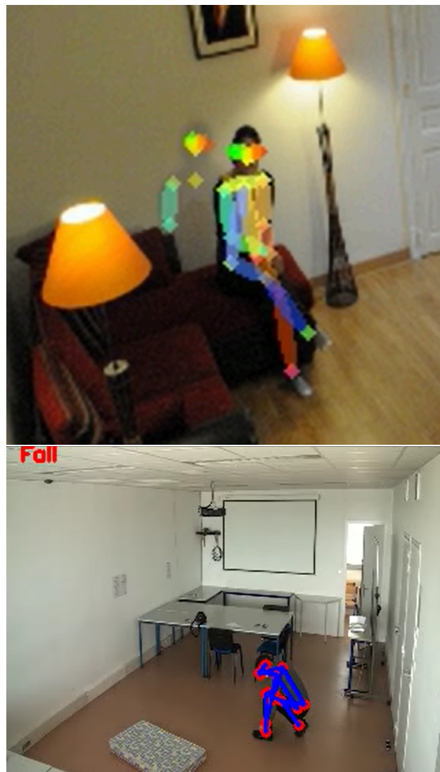
Figure 5.5: Failure cases of the proposed fall detection method. Top: incorrect human pose estimation by AlphaPose. Bottom: a failure case of STGCN-LE ( full video )
