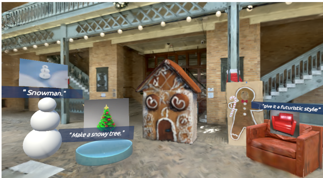
Figure 2.10: Spatial annotation tags are placed over the radiance field objects and generated objects with given instructions and preview generations.
