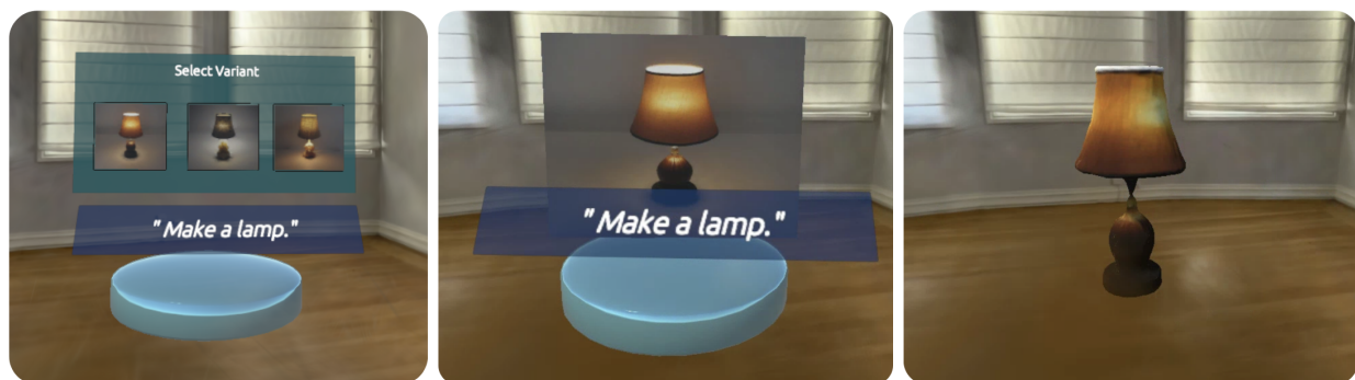
Figure 2.4: Object Generation via Prompting (Left) Object generation variations from speech input. (Center) Displaying selected generation preview as a spatial annotation. (Right) Fully processed 3D generation in the scene.
