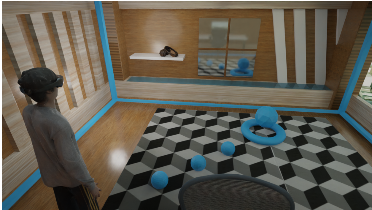
Figure 4.1: VR/AR HMD Assisted 3D Capture An interface for guiding a user to capture a NeRF dataset using head-mounted cameras and headset poses from a VR/AR headset
