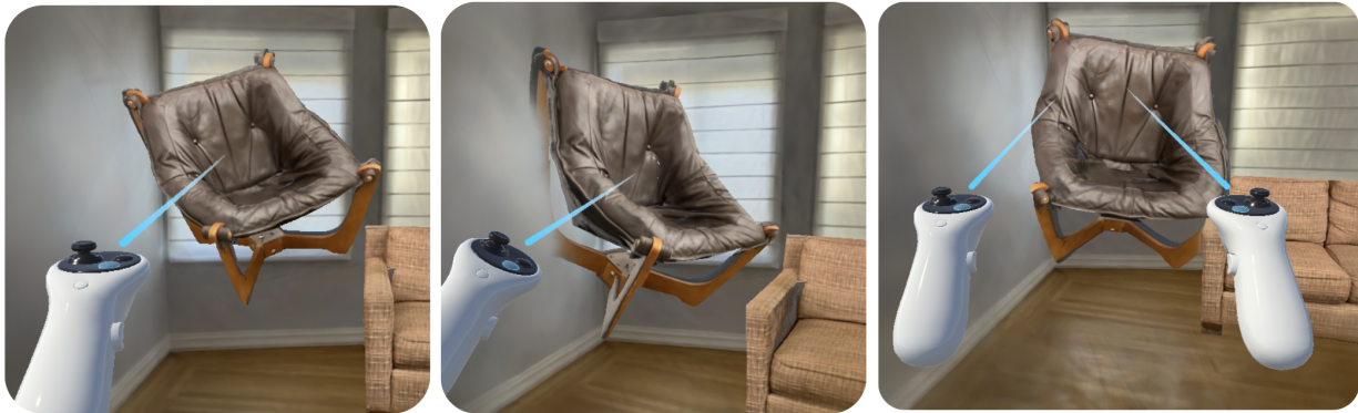
Figure 2.2: Object transformations and direct manipulations (Left) Positioning object in the scene (Center) Rotating object. (Right) Scaling object
