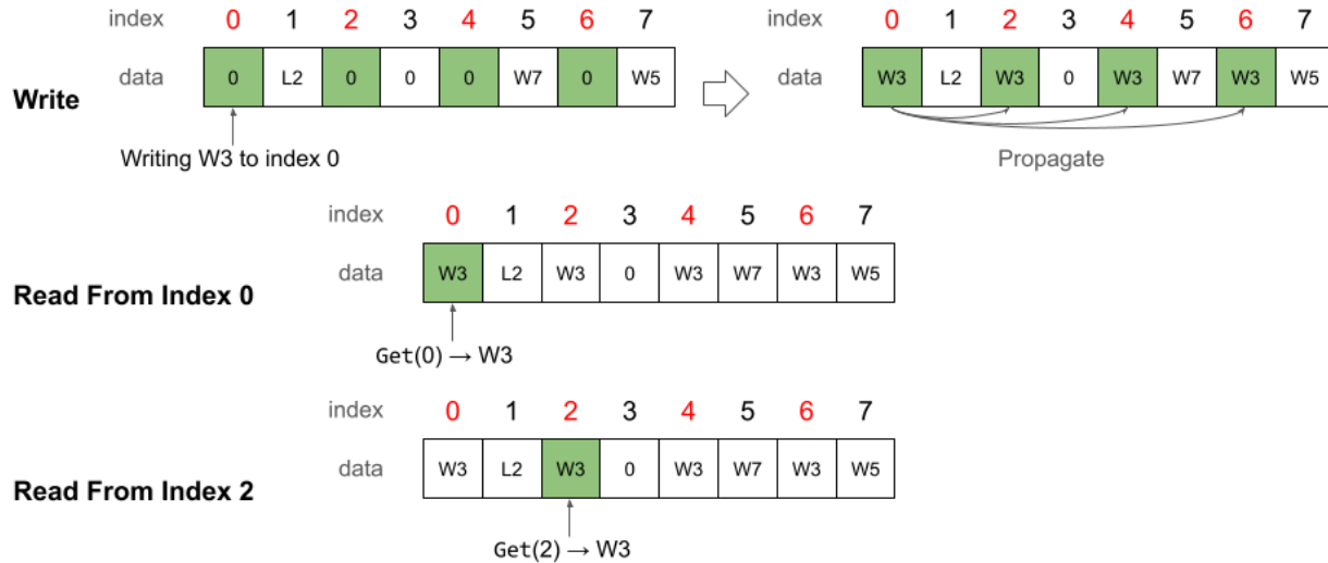
Figure 2.7: Writing to and reading from a database under the ROWM model
