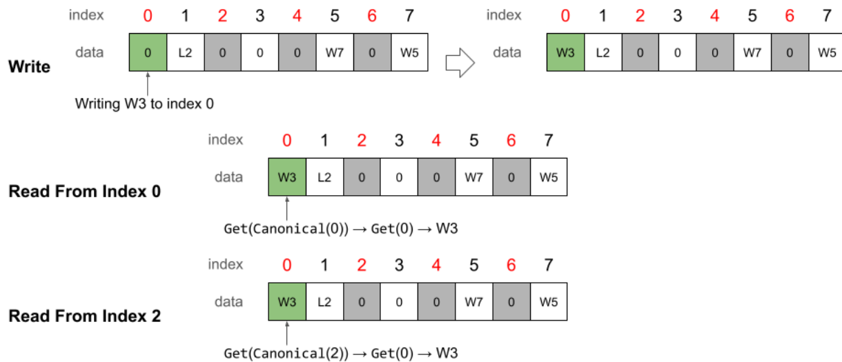
Figure 2.6: Writing to and reading from a database under the WORM model
