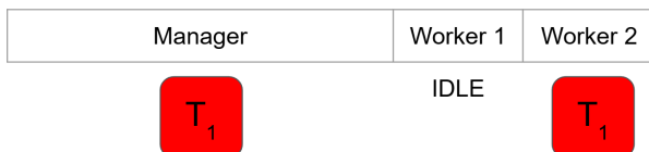
Figure 4.1.7: State of the tier solver after worker 2 finishes solving T_3 and receiving T_1 from the manager
