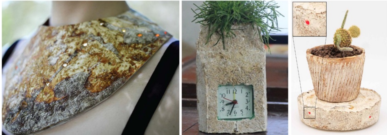
Figure 2.3: Mycelium has emerged in HCI as a popular material that can be grown and readily decomposed in backyard soil. It can be shaped and used as a substrate for conventional electronic parts. From left to right: mycelium wearable with decorative LEDs [340], mycelium clock [367], mycelium flower pot with an integrated moisture sensor and LED indicators [104].
