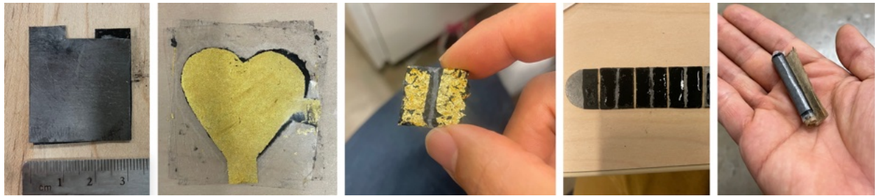
Figure 5.5: Readily fabricated in a makerspace with hand tools, Vims can take a variety of shapes and form factors.
