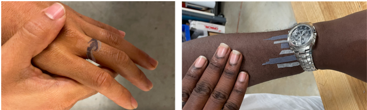
Figure 6.3: Lotio sense and react to applied lotion. Left: “Ocean Waves” ring prototype behaves as a fashionable form of personal expression. Right: “Skyscraper Skyline” prototype extends the display capabilities of a smartwatch onto the skin.
