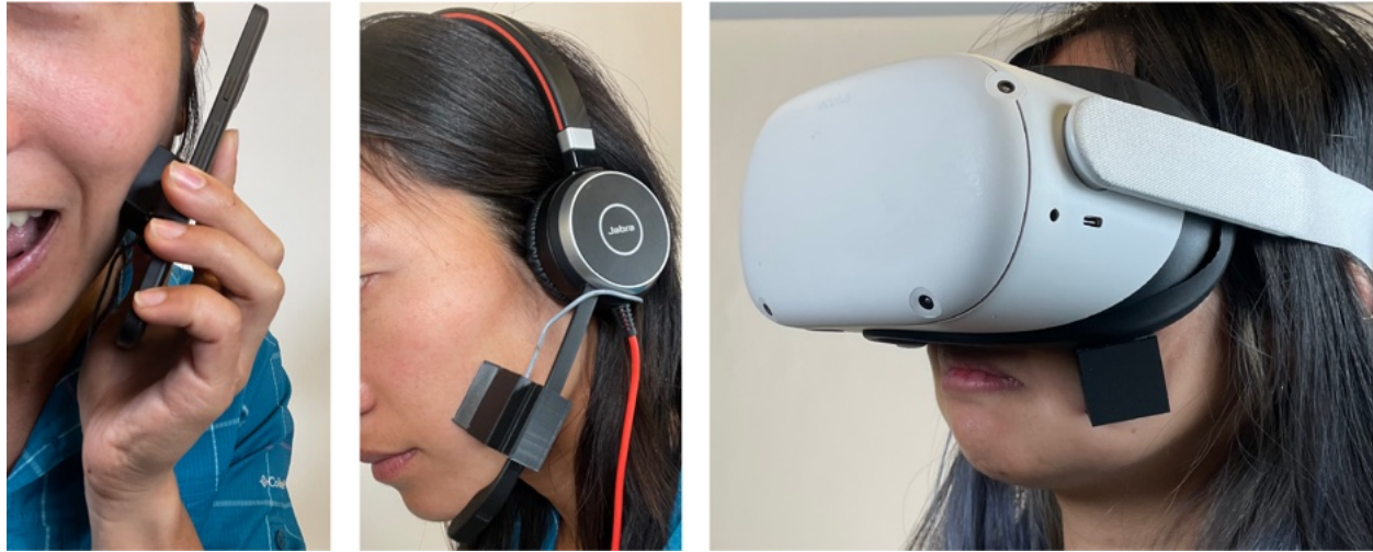
Figure 4.13: Mock-ups of Füpops electronics integrated into a cell phone, an audio headset, and a head-mounted display.
