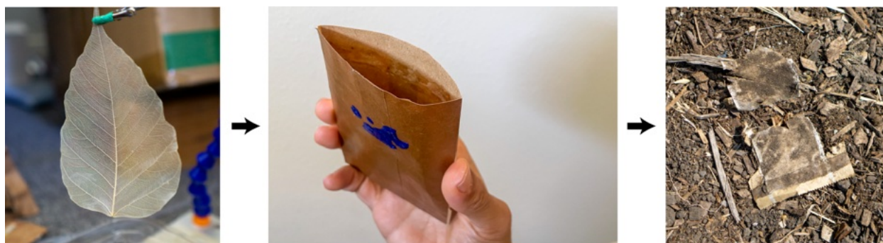
Figure 3.1: From leaf skeletons (left), I create a lightweight packaging that can wirelessly heat its contents (center) and is fully backyard-degradable (right).
