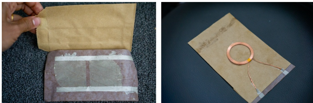
Figure 3.7: Left: Open-faced view of the leaves, silver traces, and paper packaging. Right: Reverse side of packaging showing charging coil (off-the-shelf copper coil used as stand-in for printed silver coil).
