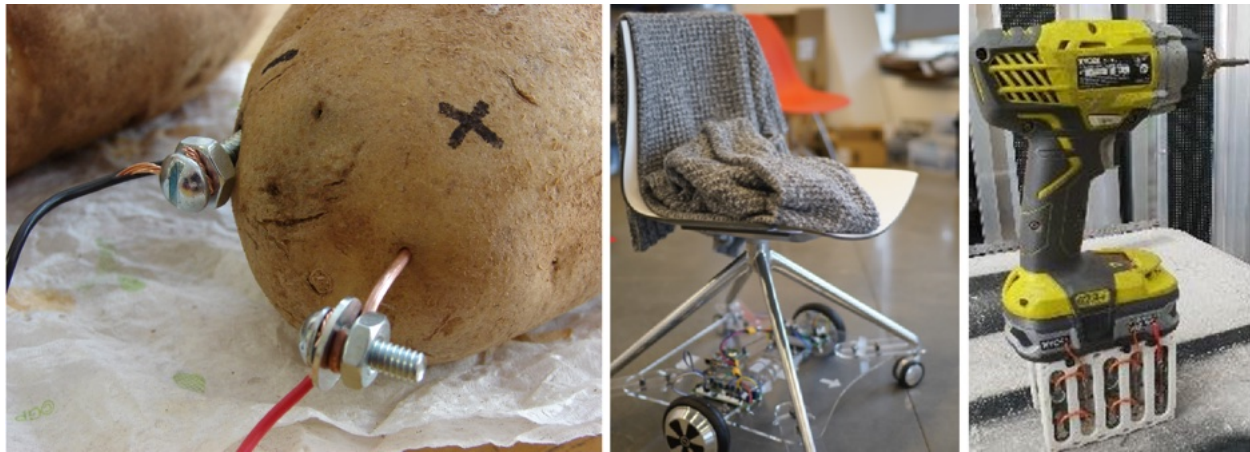
Figure 2.4: A selection of DIY-friendly electronics made from scavenging food, e-waste, and other accessible materials. From left to right: battery made from a potato with copper wire and iron nail electrodes (David R. Tribble), robotic chair made from parts from a hoverboard [210], and drill with battery pack with parts scavenged from an e-waste recycling center [350].
