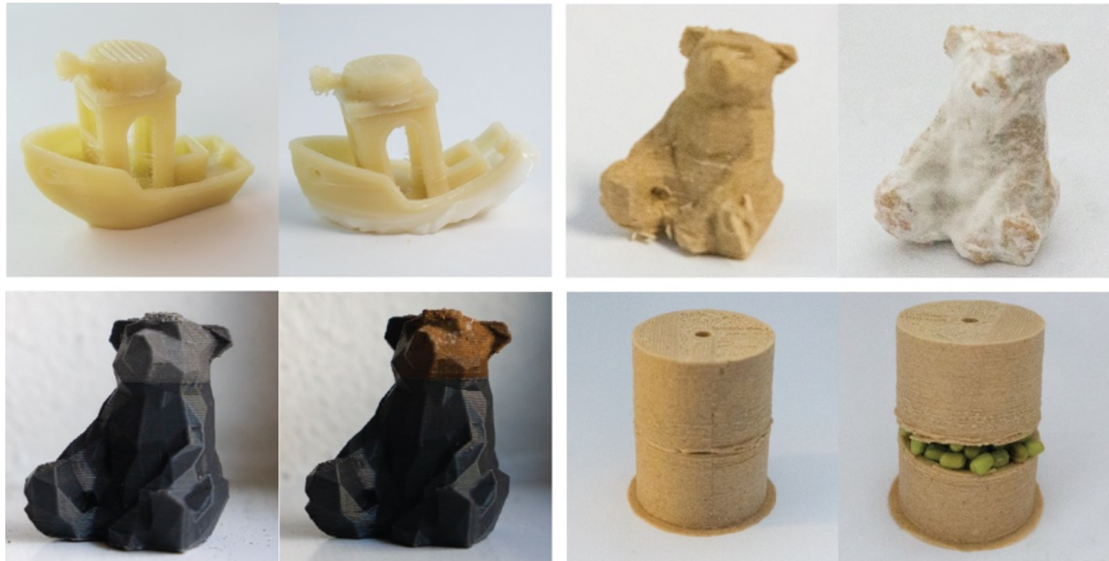
Figure 7.3: Demonstrations of different unmaking strategies. Top left: Single material printing: A PVA model is selectively dipped in water; water is absorbed and causes melting and splitting. Top right: Multi-material printing (obscured): A Timberfill wood-PLA composite shell is filled with mycelium spores; mycelium colonizes the shell material, softening it and drastically changing its appearance. Bottom left: Multi-material model printing (overt): A model comprising solid PLA for the body and iron-PLA composite for the head; when exposed to salt water, the head selectively rusts. Bottom right: Obscured multi-material printing + counter-stable mechanical design: A wood-PLA composite shell is filled with hydrated mung beans; the sprouting of the mung beans causes cleavage along a pre-defined weak layer in the cylinder.
