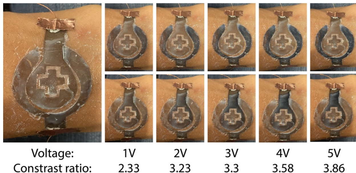
Figure 6.10: Visual clarity of Lotio under an applied voltage of 1 to 5V. In the top row, the positive voltage is connected to the top part of the design with the bottom part of the design grounded. In the bottom row, the voltage is reversed.
