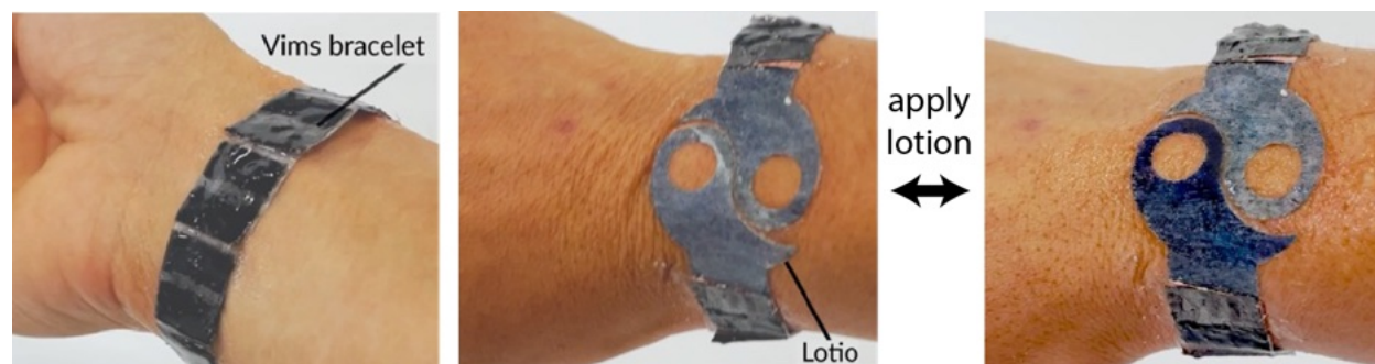
Figure 6.17: A 100% backyard-degradable wearable. Vims are chained in series as a bracelet and contact the electrodes of a simple Lotio design. When lotion is applied as an electrolyte, parts of the design change color, revealing a hidden message (in this case, “CHI”).
