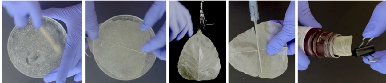
Figure 3.5: Fabrication process of leaf heating elements. From left to right: a chitosan jelly is stirred by hand, a leaf skeleton is dipped into the jelly, the leaf is hung to dry, the leaf is cut by hand with scissors into patches, and then the leaf is dipped into a silver nanowire solution.
