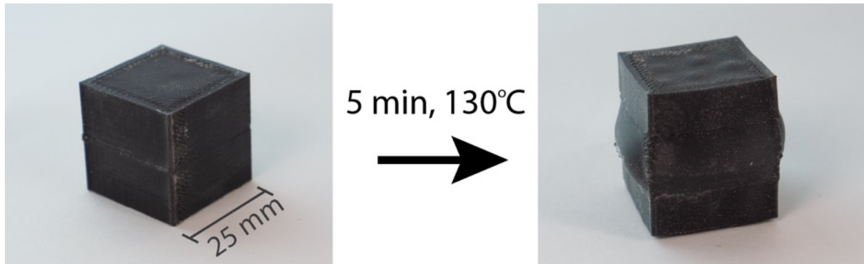
Figure 7.6: A pre-defined section of a PLA cube bulges upon heating.
