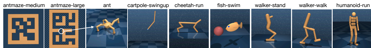
Figure 4.6: Tasks for our empirical evaluation. We include the challenging AntMaze navigation tasks from D4RL [10] and low (1-DoF) to high (21-DoF) dimensional locomotion tasks from DeepMind Control Suite [11].
