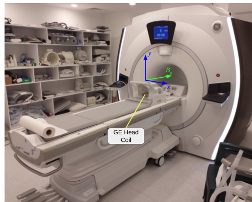
Figure 3.1: The GE Discovery MR750W 3.0T Scanner is used in this project. Installed is the GE Head Coil that is used for transmit and receive signal throughout this project on the small spherical phantom. The scanner features a 3 Tesla B_0 magnet, with linear gradients for shimming and scanning, all housed within the bore of the machine (the donut-looking section of the machine). There are no higher order shims included with this scanner. The \vec{B}_0 is depicted and is aligned with the z direction of the scanner. The effective \vec{B}_1 field is in the transverse ( x - y ) plane.
