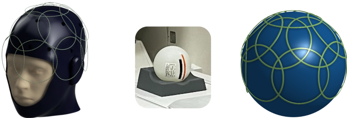
Figure 3.4: From left to right: the idealized headcap of 15 integrated Rx and Shim coils for use in the TMS-EEG-fMRI research work, reproduced from Maravilla[11]. The ball phantom used to generate background field map. The simulated ball phantom with an array of 15 coils placed around it in the same configuration as the the Rx Headcap.
