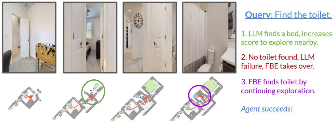
Figure 70: Tolerance to LLM failures. An example rollout of LFG compensating for LLM failure. FBE takes over in this case and eventually succeeds, whereas the Greedy agent fails.
