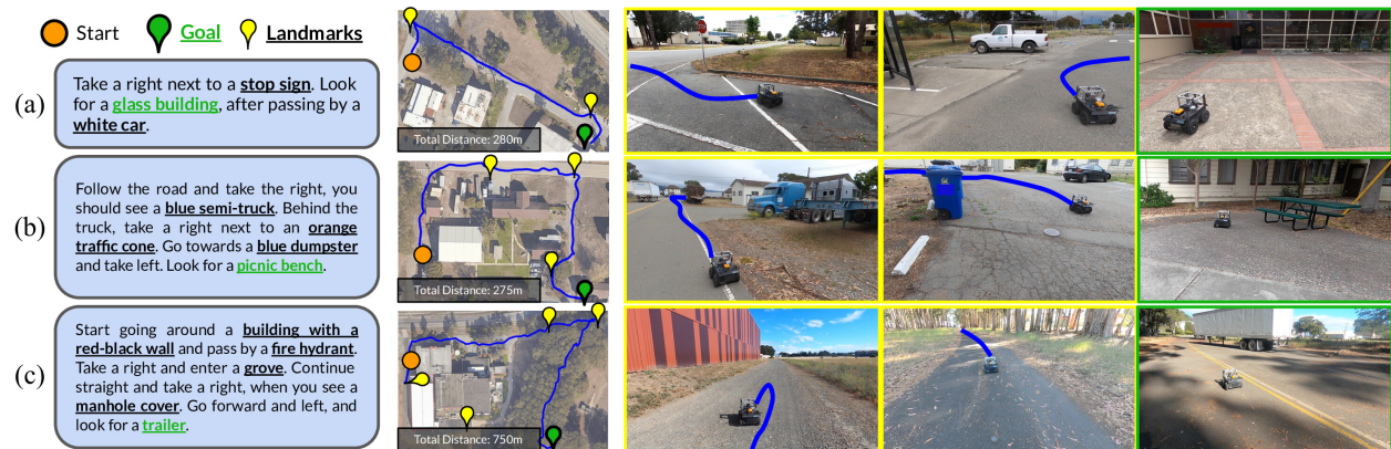
Figure 52: Qualitative examples of LM-Nav in real-world environments executing textual instructions (left). The landmarks extracted by LLM (highlighted in text) are grounded into visual observations by VLM (center; overhead image not available to the robot). The resulting walk of the graph is executed by VNM (right).
