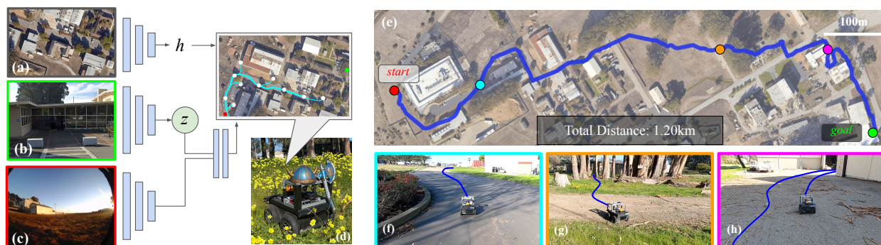
Figure 14: Kilometer-scale autonomous navigation with ViKiNG: Our learning-based navigation system takes as input the current egocentric image (c), a photograph of the desired destination (b), and an overhead map (which may be a schematic or satellite image) (a) that provides a hint about the surrounding layout. The robot (d) uses learned models trained in other environments to infer a path to the goal (e), combining local traversability estimates with global heuristics derived from the map. This enables ViKiNG to navigate previously unseen environments (e), where a single traversal might involve following roads (f), off-road driving under a canopy (g), and backtracking from dead ends (h).
