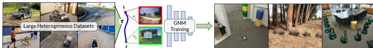
Figure 29: A general navigation model to drive any robot. By training on diverse, heterogeneous datasets, a single “omnipolicy” can control a variety of robots in challenging environments, including new robots, without any robot-specific data collection.
