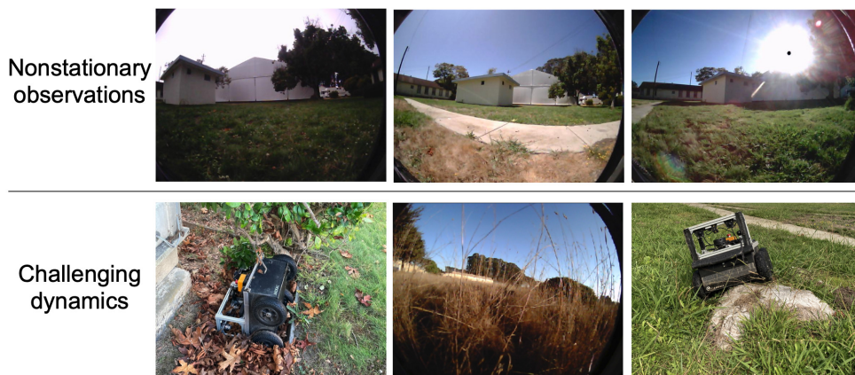
Figure 2: Challenges with Real-World Navigation: (Top) Three observations taken from exactly the same position at different times of day exhibit large differences. (Bottom) While tall grass and inclined rocks are traversable, a hole filled with dry leaves is not. These examples highlight the challenges with geometric reasoning about traversability.
