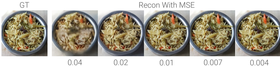
Figure C.1: Comparison of reconstructed image quality at varying MSE thresholds. The ground truth (GT) image is displayed on the left, followed by reconstructions at different MSE thresholds (0.04, 0.02, 0.01, 0.007, and 0.004), showing progressive improvement in fidelity as the threshold decreases.
