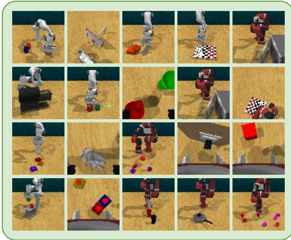
Figure E.4: A single autoregressive video model is trained on 30 tasks for the Franka Panda and 23 tasks for the ReThink Robotics Sawyer, using 16 \times 16 VQCodes and a context length of 4, with frame skip 4.
