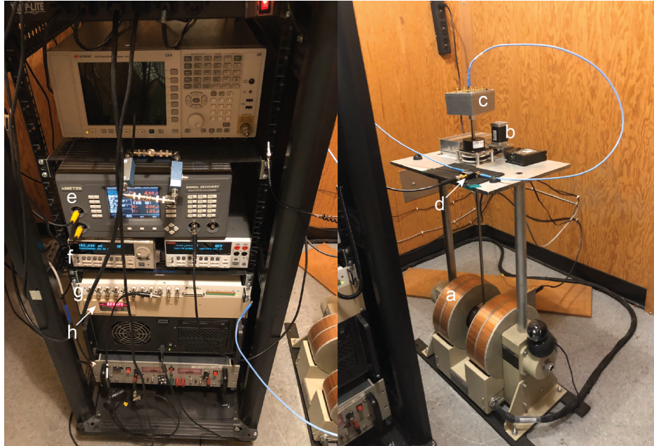
Figure A.3: a, Electromagnet capable of generating up to 0.35 T. b, Applied motion angle rotation motor assembly. c, Current box for input RF signal. d, Bias tee. e, Signal Redovery 7270 DSP Lock-in amplifier by AmTek. f, Keithley 6221A AC/DC current source. g, DAQ card. h, Gaussmeter. i, Electromagnet powersupply by Kepco.
