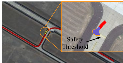
Figure 2.4: Our algorithm is applied to assure safety in potential runway incursion scenarios. Once the ground vehicle is determined to have crossed a designated safety threshold, the aircraft is cleared to land.
