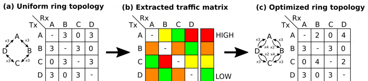
Figure 1.2: (a) Initial uniform ring topology. (b) Traffic matrix extracted from a specific application showing the relative amount of transmitted data. (c) New ring topology optimized for the extracted traffic matrix.
