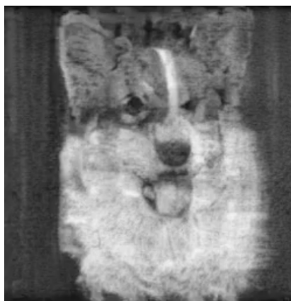
Figure 4.2: A spectrogram of an audio clip that sounds like a dog barking and looks like a corgi [376].
