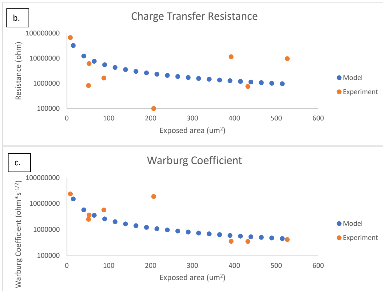
Figure 3.5 a. Double layer capacitance fit for tungsten microprobe EIS data as a function of exposed electrode area. b. Charge transfer resistance fit for tungsten microprobe EIS data as a function of exposed electrode area. c. Warburg coefficient fit for tungsten microprobe EIS data as a function of exposed electrode area
