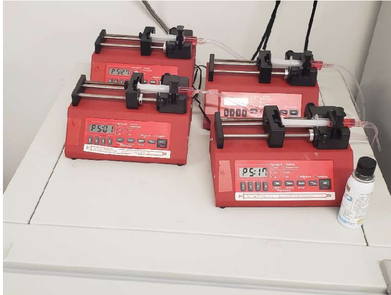
Figure 4.1 Syringe pumps were placed on top of incubator to avoid contamination of the chamber. Tubing was fed through the cord port in the side of the incubator.
