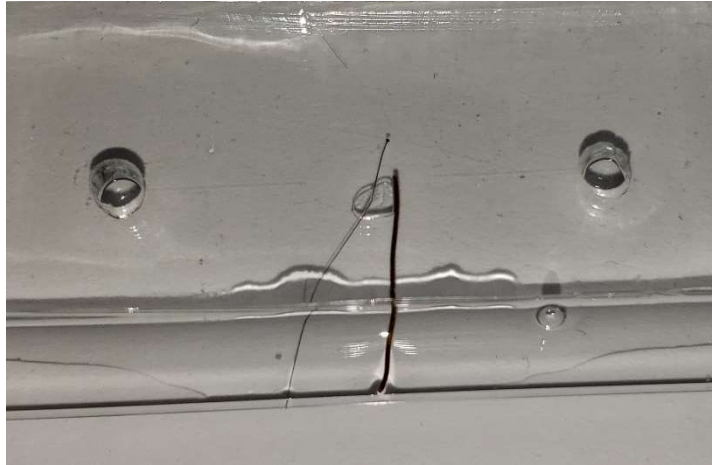
Figure 2.8. Microfluidic chamber with unsuccessful PDMS sealing (backfilled)
