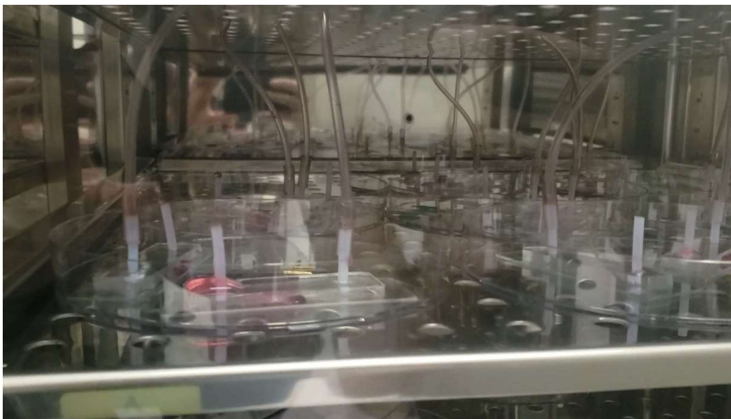
Figure 4.2 Syringe pump tubing was connected to microfluidic chambers inside of the incubator. Microfluidic chambers were transported in tissue culture polystyrene dishes to reduce contamination.
