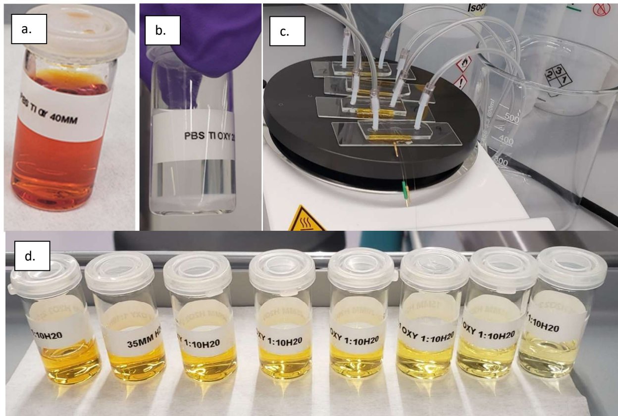
Figure 2.11. Colorimetric hydrogen peroxide concentration quantification a. 2:1 PBS/H 2 O 2 : Titanium oxysulfate solution. b. 20:1 PBS/Peroxide: Titanium oxysulfate solution. c. H 2 O 2 aging setup. H 2 O 2
