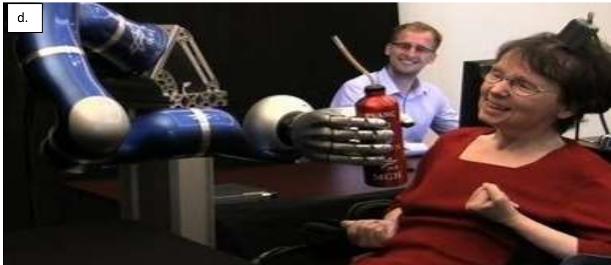
Figure 1.1 a. Implantable deep brain stimulator technology for Parkinson's treatment.[17] b. Thought-to-text conversion technology for non-verbal patients.[3] c. Schematic of brain machine interface for robotic limb control.[18] d. Human trial of brain machine interface for robotic limb control.[2]
