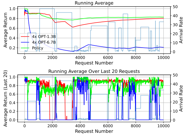
Figure 6. Running total and windowed average over the last 20 requests of performance on the unpredictable workload. The arrival rate at each step is also shown.
