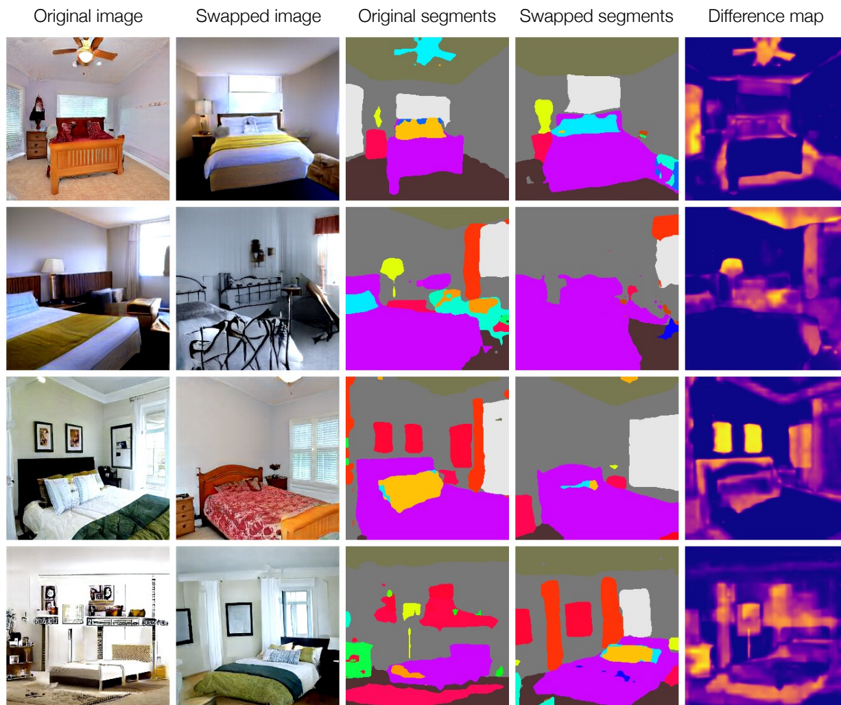
Figure 2.20: Style swapping with StyleGAN: We show randomly sampled untruncated StyleGAN images before and after style swapping at layer 4, attaining an FID of 5.04 and layout consistency of 55.3%. The difference map shows the normalized KL divergence of the predicted per-pixel logits before and after swapping.
