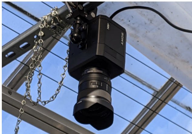
Figure 6.2: Overhead Camera: The Sony SNC-VB77 camera is used to monitor the AlphaGarden. It's characteristics include a 35mm sensor, a low aberration lens, and higher than 4K resolution to allow for crisp and clear images for monitoring.
