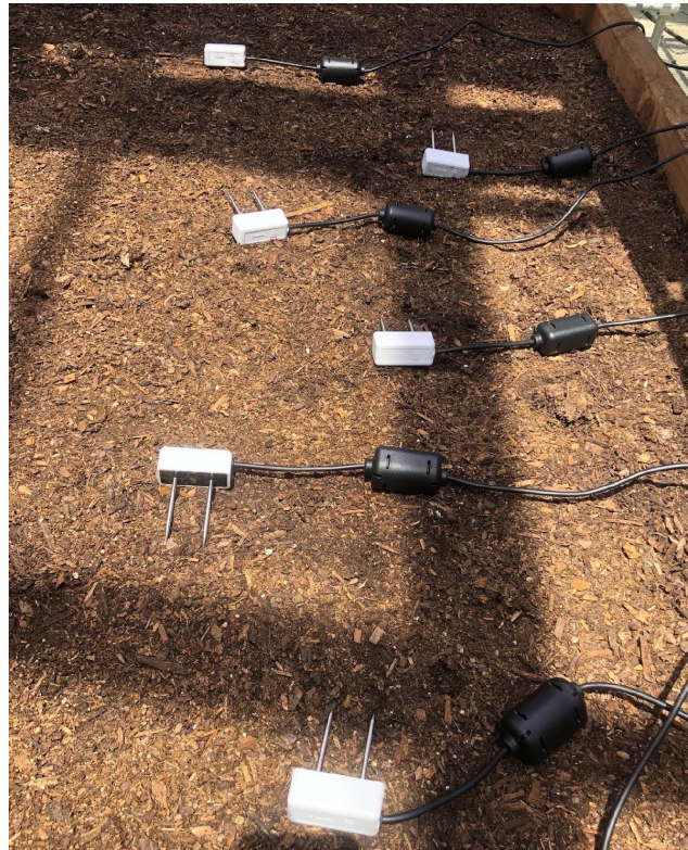
Figure 6.4: Moisture Sensors: The TEROS 10 sensors are laid throughout the garden bet to measure and model soil metrics and dynamics.
