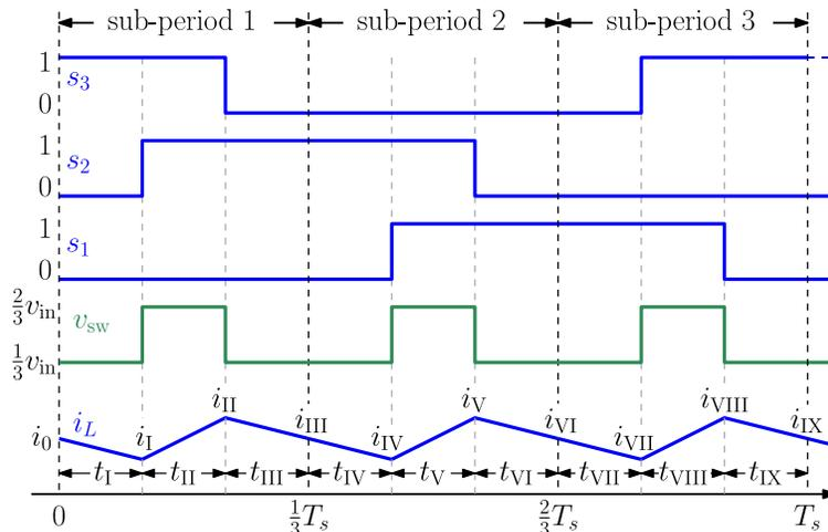
Figure 4.2: Switching signals  $s_k$ , switching node voltage  $v_{sw}$ , and inductor current  $i_L$  for a 4-level FCML converter operating in mode 2. The switching phases occurring in each sub-period and the value of the inductor current at the end of each switching phase are annotated with roman numerals.
