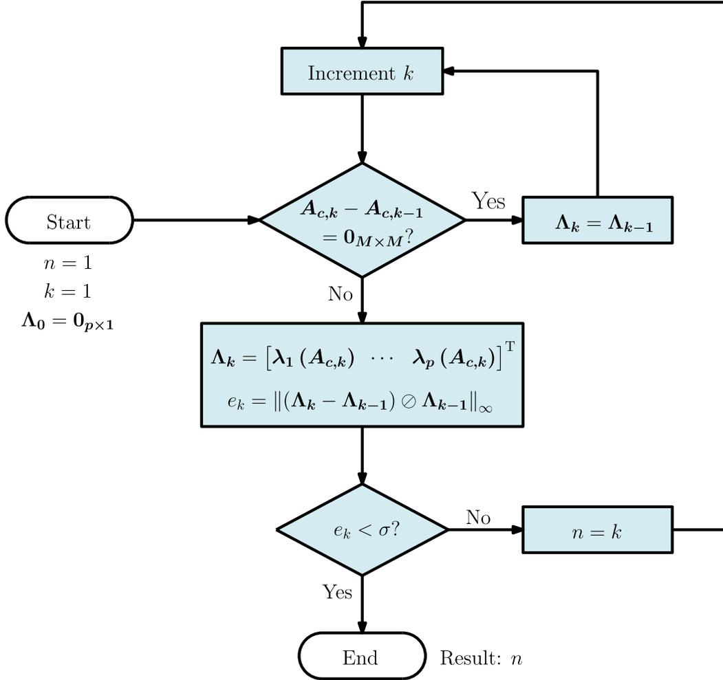
Figure 3.10: Flowchart depicting the procedure proposed in this section to determine the minimum number of inductor current harmonics required to capture the capacitor voltage dynamics.
