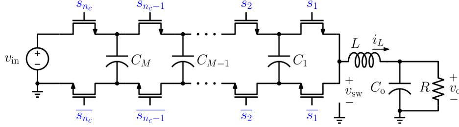
Figure 2.3: Schematic drawing of an  $N$ -level FCML converter with  $n_c = N - 1$  complementary switch pairs and  $M = N - 2$  flying capacitors.
