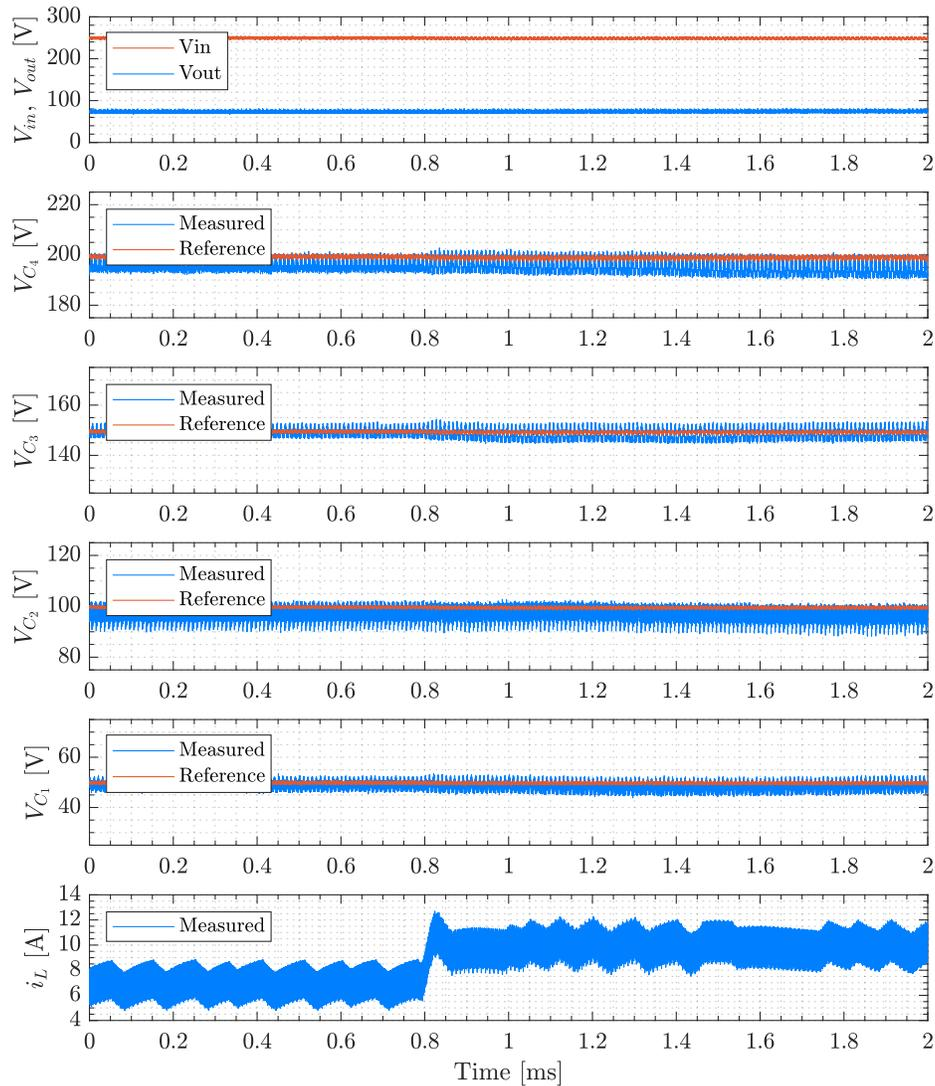
Figure 2.15: Measured capacitor voltage and current response during a step change in the current reference  $i_{\text{ref}}$  from 7 A to 10 A at  $v_{\text{in}} = 250$  V. The current control bandwidth is set to 10 kHz. The flying capacitor voltages are undisturbed during the load current transient, verifying that the capacitor voltages naturally reject the common-mode duty ratio used to control current.
