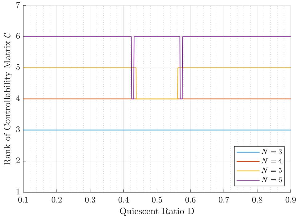
Figure 3.26: Rank of the controllability matrix  $\mathcal{C}$  associated with the small-signal system of (3.58) as a function of the quiescent duty ratio  $D$  for a 3-level, 4-level, 5-level, and 6-level converter.
