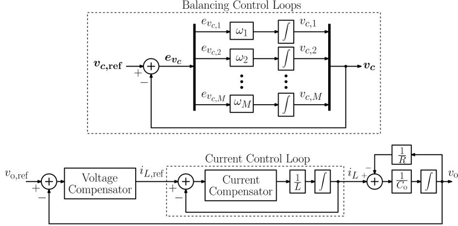
Figure 2.9: Equivalent closed-loop system after feedback linearization of the current dynamics. To ensure the balancing disturbance is rejected in practice, the current controller bandwidth should be chosen to be significantly higher than the balancing control bandwidth.
