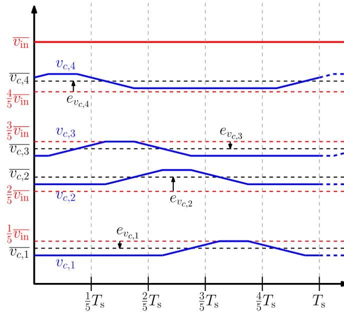
Figure 2.7: Example imbalanced capacitor voltages, shown in a timescale of one switching period. The reference capacitor voltages are respective nominal fractions of the input voltage,  $\frac{k}{n_c} V_{in}$ , shown as red lines. The signed errors associated with imbalanced voltages are indicated by arrows.
