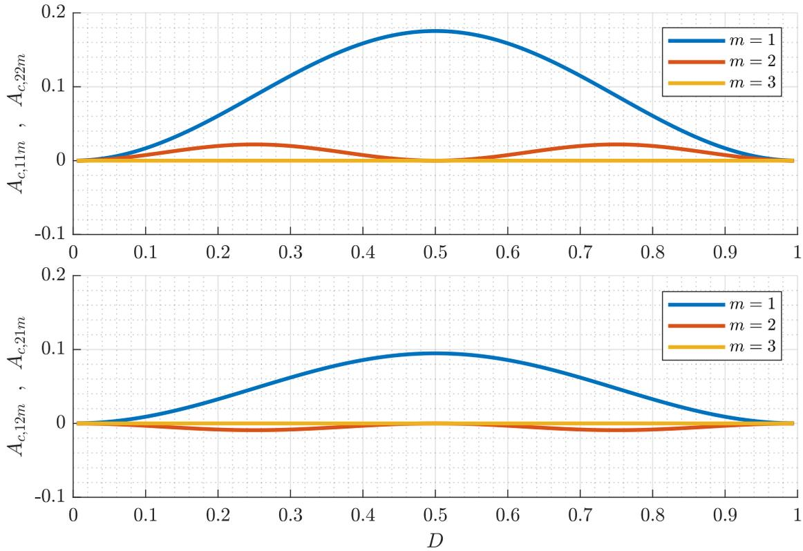
Figure 3.8: Plots of  $A_{c,klm}$  as given by (3.51) normalized to  $-\frac{\omega_0}{m\Omega_s}$  for a 4-level converter. The curves depict the contribution of different inductor current harmonics to the capacitor dynamics. For a small range of duty ratios centered at  $D = 0.5$ , the contributions of the second and third harmonics are negligible.
