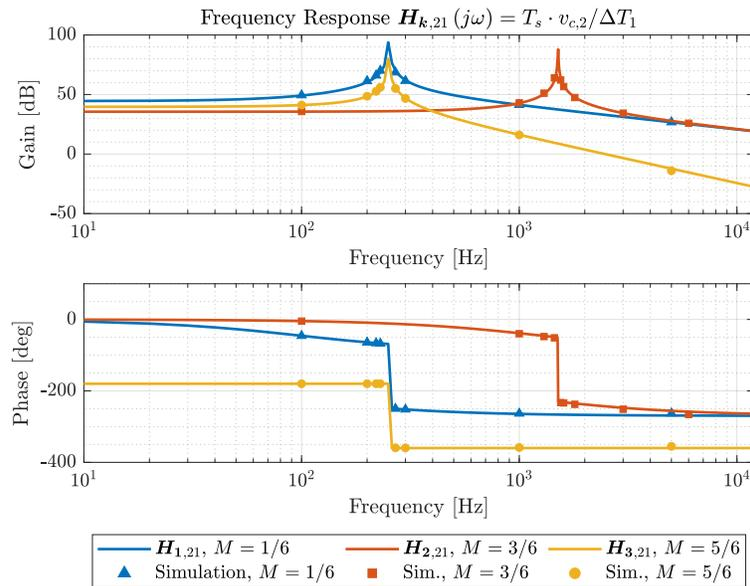
Figure 4.11: Comparison of simulated frequency response of capacitor voltage  $v_{c,2}$  to perturbations in  $\Delta T_1$  to the theoretical response  $\mathbf{H}_{k,21}$  obtained from (4.34). The simulation results agree with the theoretical frequency response in all operating modes up to a tested bandwidth of 5 kHz.
