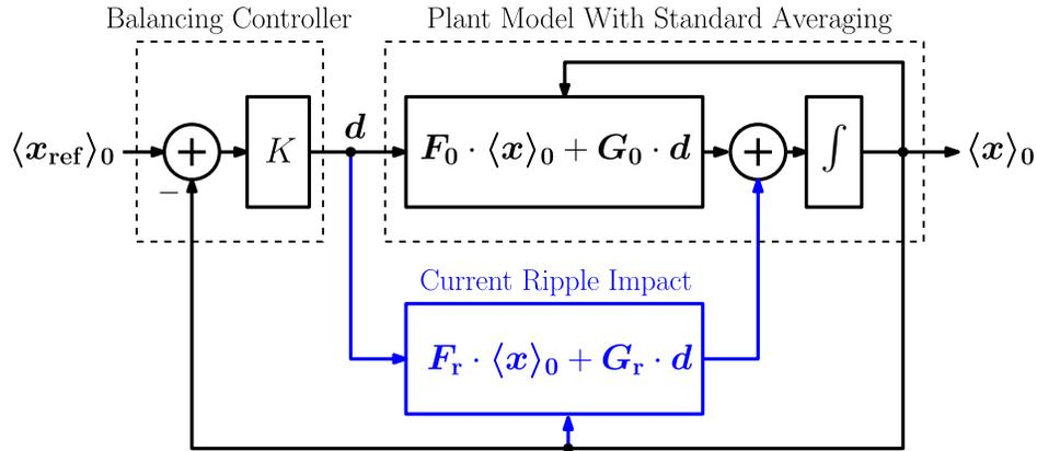
Figure 3.17: Block diagram representation of the closed-loop small-signal system. The additional plant dynamics captured in the generalized averaged model are highlighted and can destabilize active-balanced systems designed around the standard averaged model in light-load conditions.
