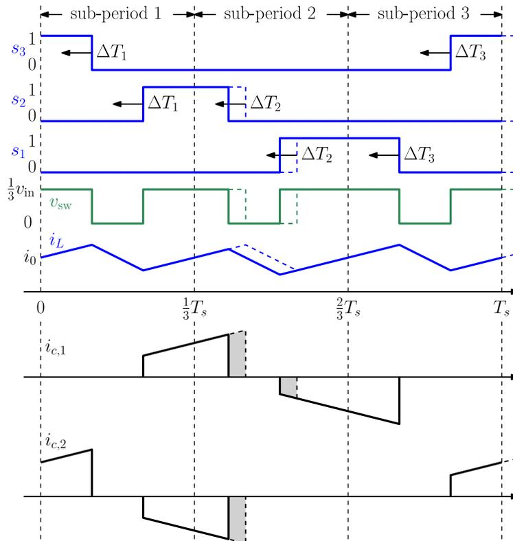
Figure 4.6: Converter waveforms illustrating the small-signal capacitor current response in operating mode 1 to a perturbation in the switching node voltage pulse position in sub-period 2. The small-signal impact of all perturbations is summarized in (4.23).
