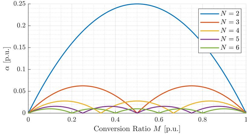
Figure 1.4: Parameter  $\alpha$  given by (1.8) plotted as a function of conversion ratio  $M$  for different level counts  $N = 2, \dots, 6$ .
