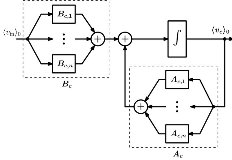
Figure 3.9: Block-diagram representation of the capacitor voltage dynamics after model-order reduction. The feedback elements model the coupling between capacitors due to each inductor current harmonic as given by (3.53).
