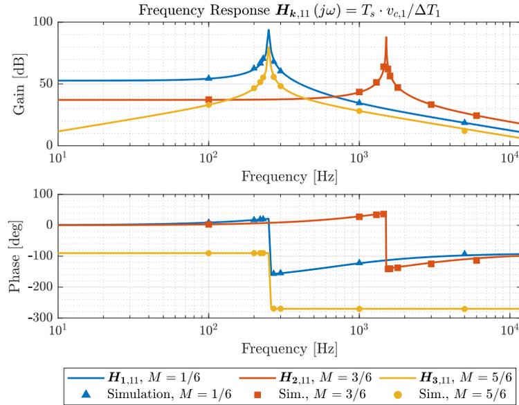
Figure 4.10: Comparison of simulated frequency response of capacitor voltage  $v_{c,1}$  to perturbations in  $\Delta T_1$  to the theoretical response  $\mathbf{H}_{k,11}$  obtained from (4.34). The simulation results agree with the theoretical frequency response in all operating modes up to a tested bandwidth of 5 kHz.
