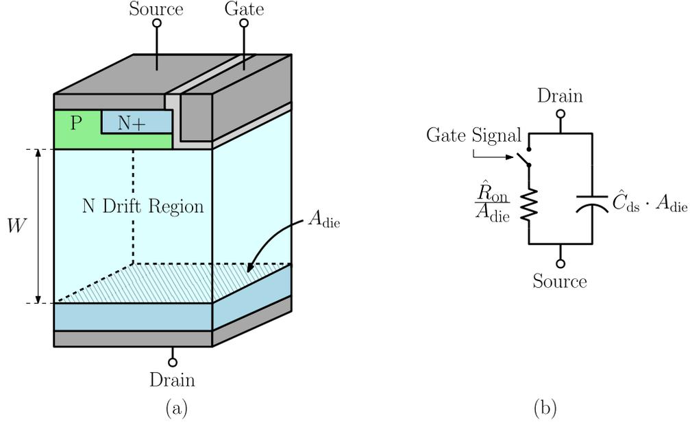
Figure 1.6: (a) Canonical vertical power semiconductor model used in [34, 35] to derive the voltage scaling characteristic of (1.14); (b) Equivalent circuit model of power semiconductor device, modeling parasitic per-unit-area on-state resistance  $\hat{R}_{\text{on}}$  and per-unit-area drain-to-source capacitance  $\hat{C}_{\text{ds}}$ .
