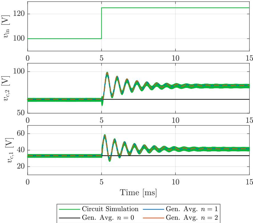
Figure 3.14: Simulated and modeled capacitor voltage responses for a 4-level FCML converter operating at  $D = 0.50$ , varying the total numbers of harmonics modeled  $n$ . The model with  $n = 1$  accurately captures the step-transient response. In the circuit simulation and model,  $L = 10 \mu\text{H}$ ,  $C = 8.8 \mu\text{F}$ ,  $R = 5 \Omega$ ,  $R_s = 0.3 \Omega$ , and  $f_s = 100 \text{ kHz}$ . The line voltage is stepped from 100 V to 125 V.
