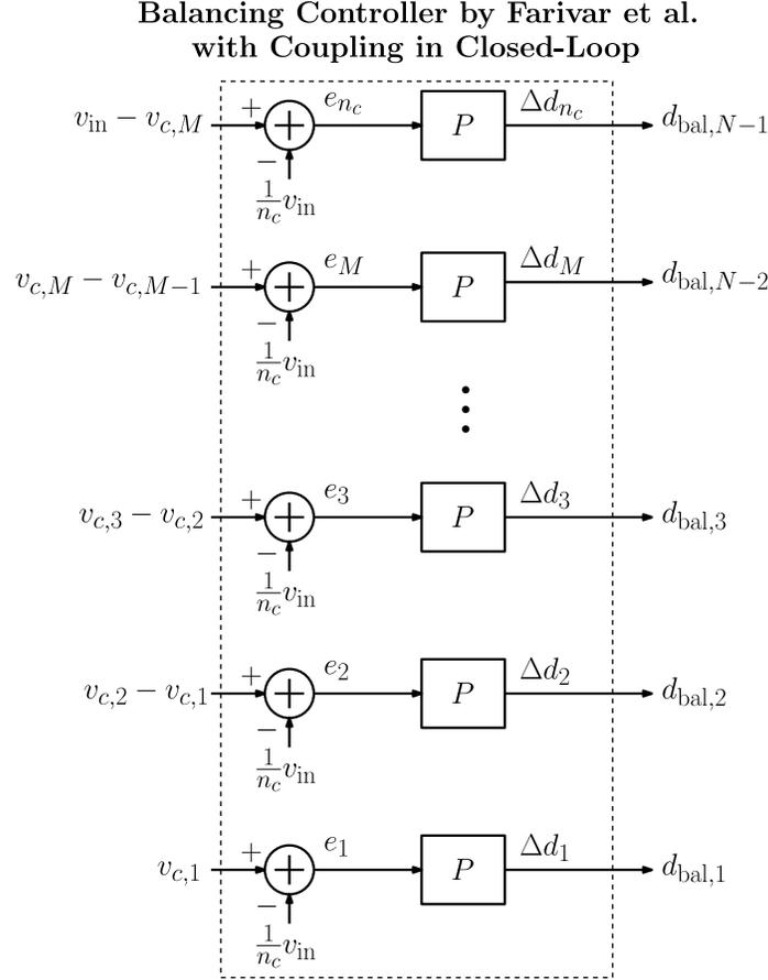
Figure 2.20: Structure of the active balancing controller proposed in [108, 111–113]. As shown in (2.56), this balancing controller results in coupled capacitor voltage dynamics and forces low-bandwidth operation in practice.
