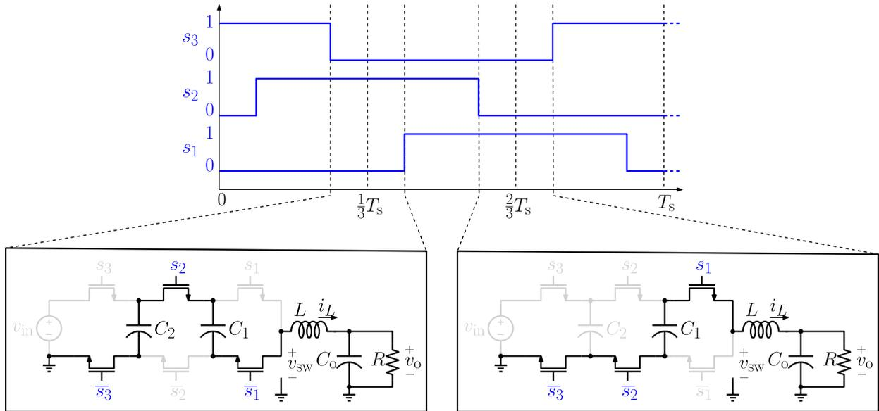
Figure 1.11: Switching signals under PS-PWM for a 4-level FCML converter, highlighting the circuit states in two switching phases. In each switching phase, a maximum of two flying capacitors are connected in series with the inductor.
