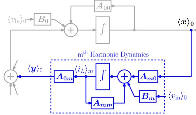
Figure A.1: Block diagram representation of the feedback dynamics corresponding to the  $m^{\text{th}}$  harmonic coefficient of the inductor current.
