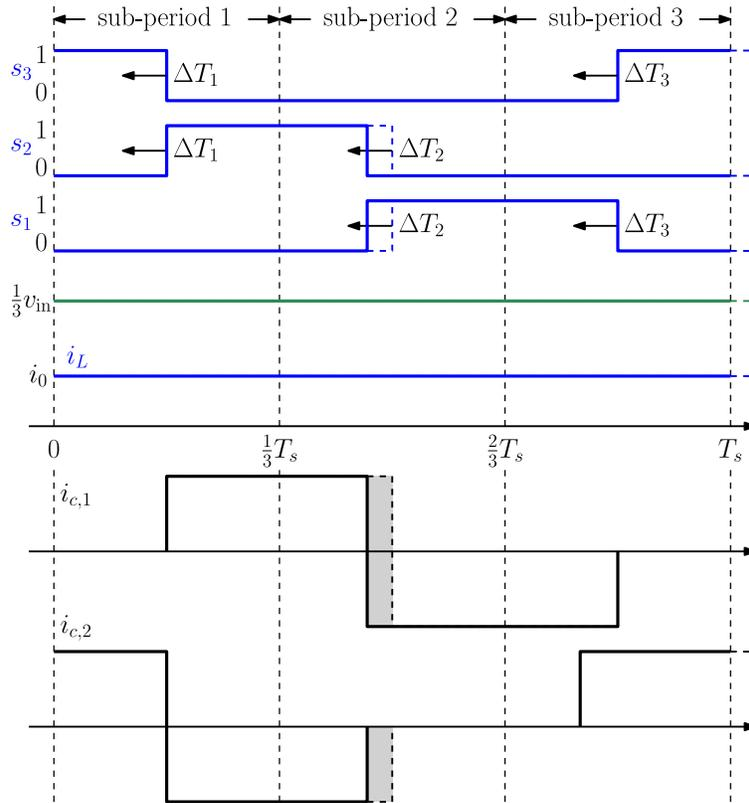
Figure 5.1: Converter waveforms illustrating the small-signal capacitor current response when  $M = 1/3$  to a perturbation in the switching signal edges occurring in sub-period 2.
