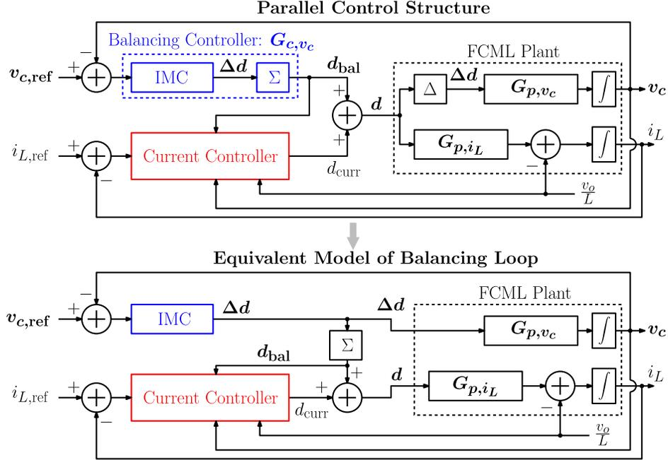
Figure 2.5: Parallel control structure and an equivalent model of the controller. The flying capacitor plant naturally rejects the common duty ratio term  $d_{\text{curr}}$  applied to all switches, as shown in the equivalent model.
