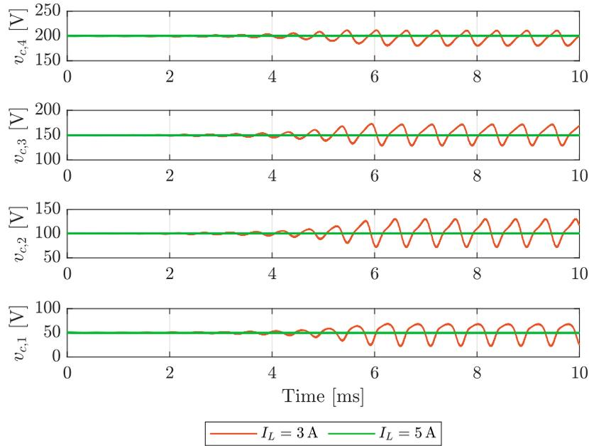
Figure 3.18: Simulated capacitor voltages for a 6-level FCML converter implementing the parallel active balancing controller of [96] at two different average load current conditions. The closed-loop system is destabilized at light-loads by the contribution of the current ripple. In this experiment,  $v_{\text{in}} = 250$  V,  $D = 0.25$ ,  $L = 10 \mu\text{H}$ ,  $C = 8.8 \mu\text{F}$ ,  $R_s = 0.3 \Omega$ , and  $f_s = 100$  kHz.
