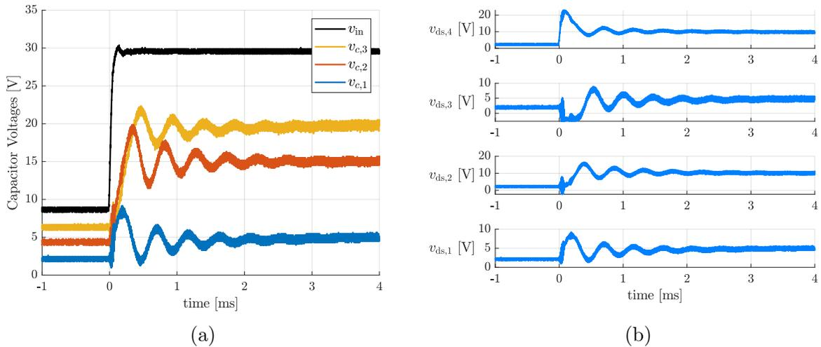
Figure 1.13: (a) Measured waveforms of Fig. 1.12, showing the underdamped capacitor voltage behavior in a timescale of 4 ms after the input voltage step; (b) Off-state switch drain-source voltages  $v_{ds}$ , highlighting the excessive voltage observed across switch pair  $s_4$ .
