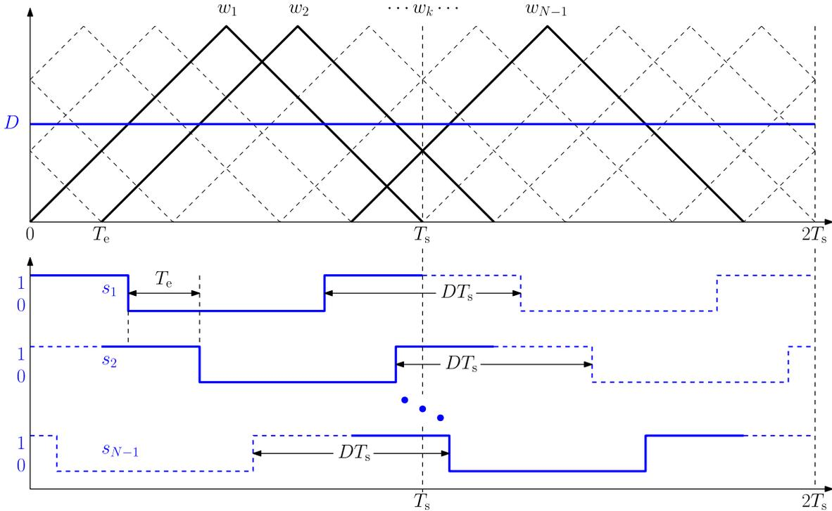
Figure 1.2: Carriers  $w_k$  and switching signals  $s_k$  ( $k \in \{1, 2, \dots, N - 1\}$ ) corresponding to symmetric Phase-Shifted Pulse Width Modulation (PS-PWM).
