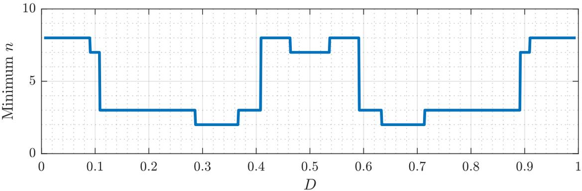
Figure 3.15: Minimum number of inductor current harmonics required to model capacitor voltage dynamics in a 6-level converter, determined from the procedure outlined in Section 3.3. The converter parameters used in this example are  $L = 10 \mu\text{H}$ ,  $C = 8.8 \mu\text{F}$ ,  $R_s = 0.3 \Omega$ ,  $V_{\text{in}} = 80 \text{V}$ ,  $I_{\text{out}} = 5 \text{A}$ ,  $R = V_{\text{in}}D/I_{\text{out}}$ , and  $f_s = 100 \text{kHz}$ .
