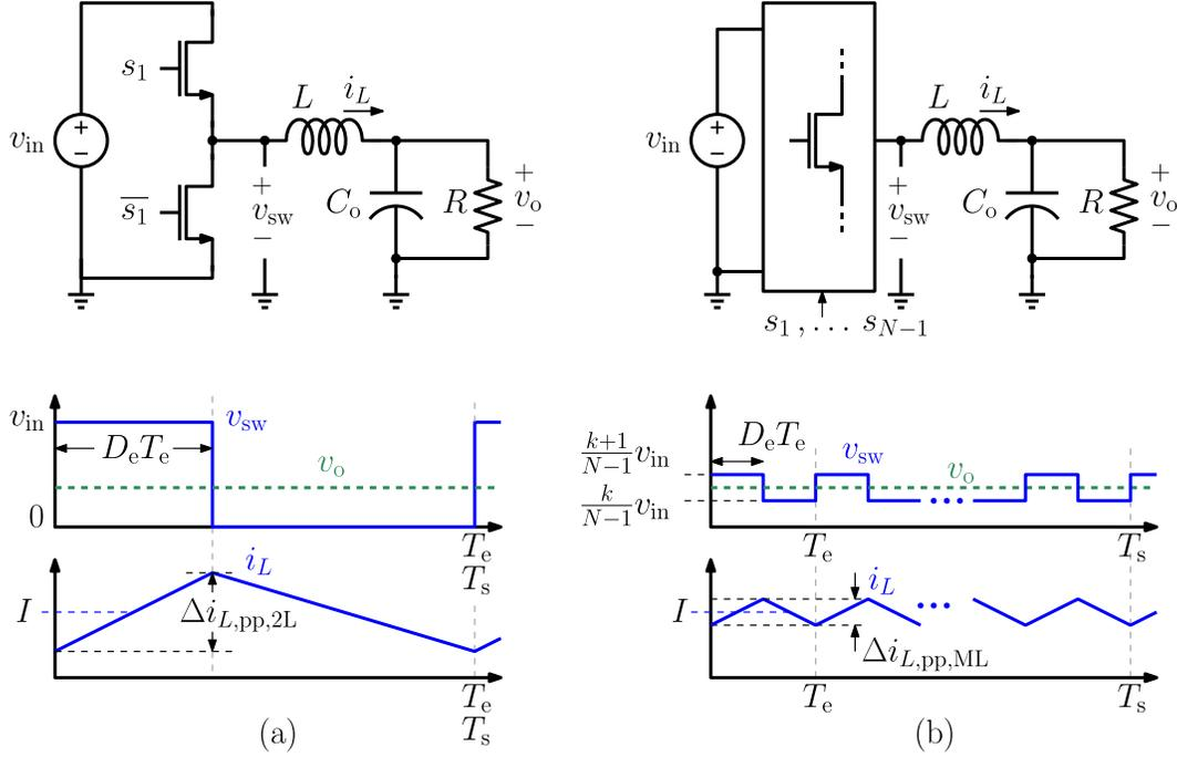
Figure 1.3: Steady-state switching node voltage  $v_{sw}$  and inductor current waveform  $i_L$  for (a) standard two-level buck converter; (b)  $N$ -level multilevel converter.
