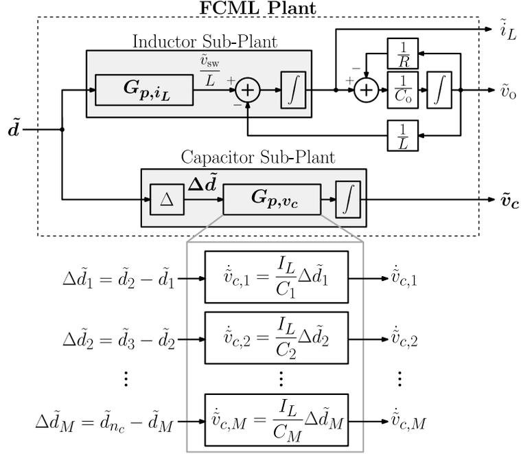
Figure 2.4: Block diagram of the small-signal averaged plant given in (2.21), highlighting the parallel inductor and capacitor sub-plants.
