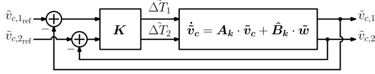
Figure 4.12: Block-diagram representation of the small-signal active balancing control loop. The controller  $\mathbf{K}$  is designed in this work to damp the natural capacitor voltage oscillations.
