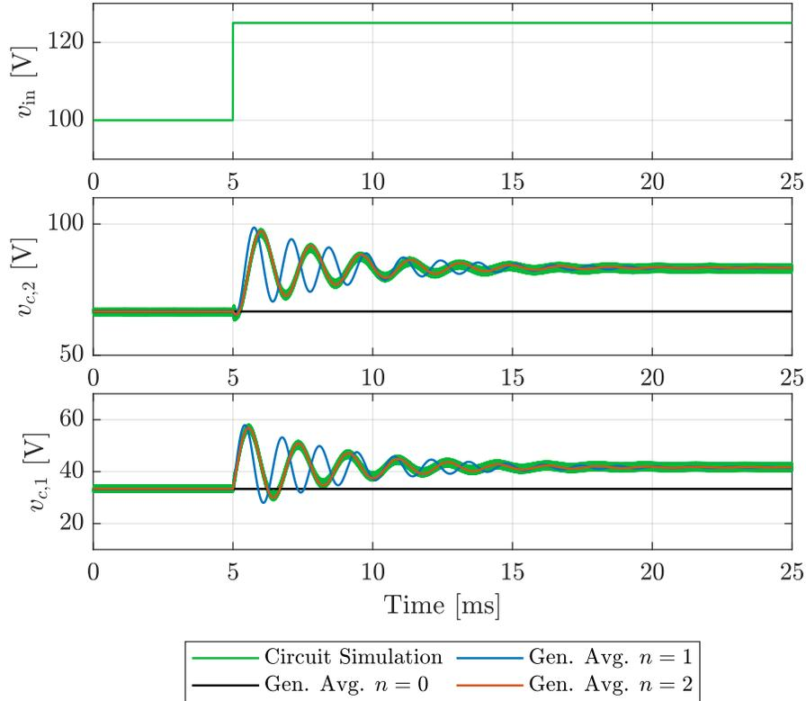
Figure 3.13: Simulated and modeled capacitor voltage responses for a 4-level FCML converter operating at  $D = 0.25$ , varying the total numbers of harmonics modeled  $n$ . The model with  $n = 2$  accurately captures the step-transient response. In the circuit simulation and model,  $L = 10 \mu\text{H}$ ,  $C = 8.8 \mu\text{F}$ ,  $R = 2.5 \Omega$ ,  $R_s = 0.3 \Omega$ , and  $f_s = 100 \text{ kHz}$ . The line voltage is stepped from 100 V to 125 V.
