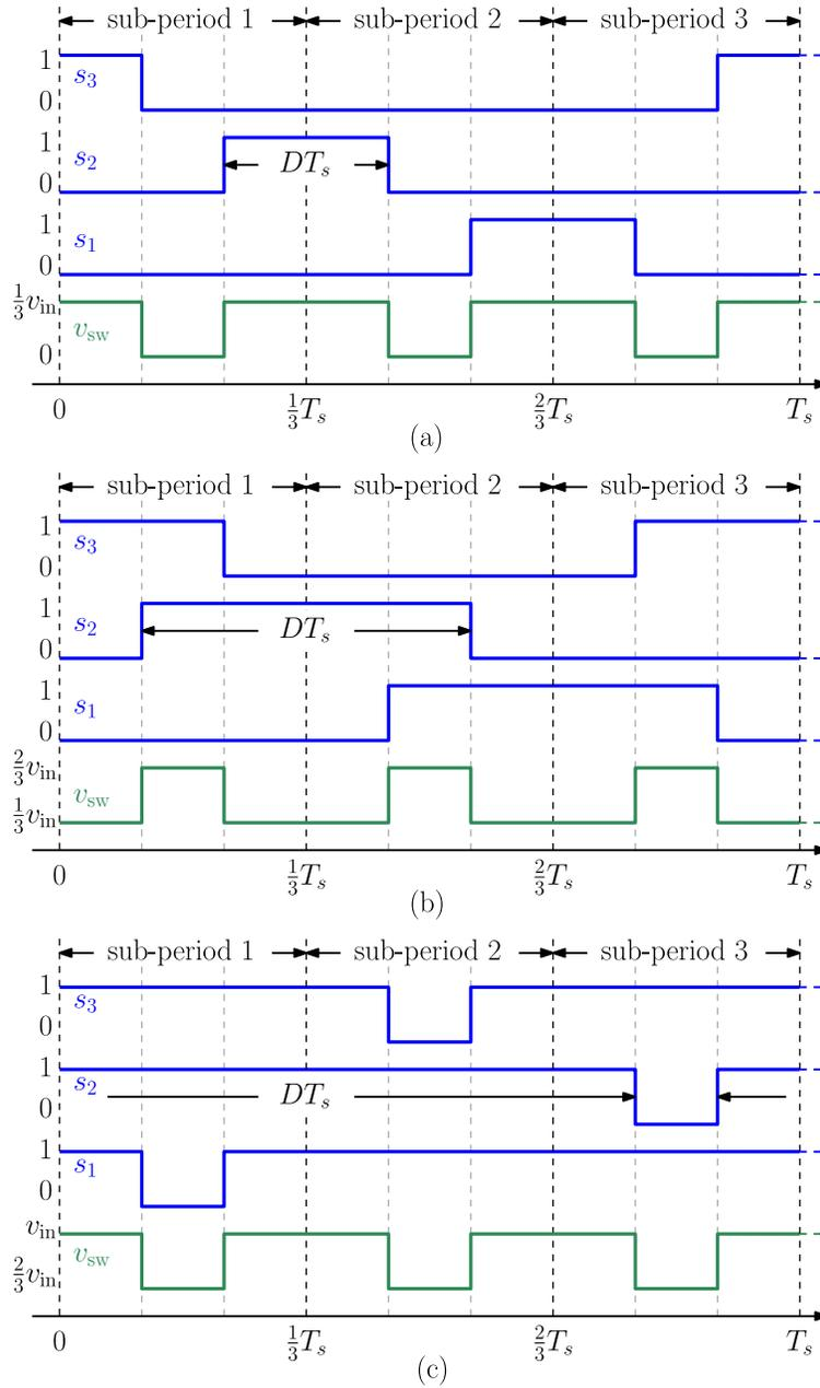
Figure 4.1: Switching signals  $s_k$  and switching node voltage  $v_{sw}$  for a 4-level FCML converter resulting from phase-shifted pulse-width modulation (PS-PWM) with duty ratio  $D$  for (a) Mode 1,  $0 < D < 1/3$ , (b) Mode 2,  $1/3 < D < 2/3$ , (c) Mode 3,  $2/3 < D < 1$ . In all three operating modes, the average value of the switching node voltage and the output voltage are equal to  $D v_{in}$ .
