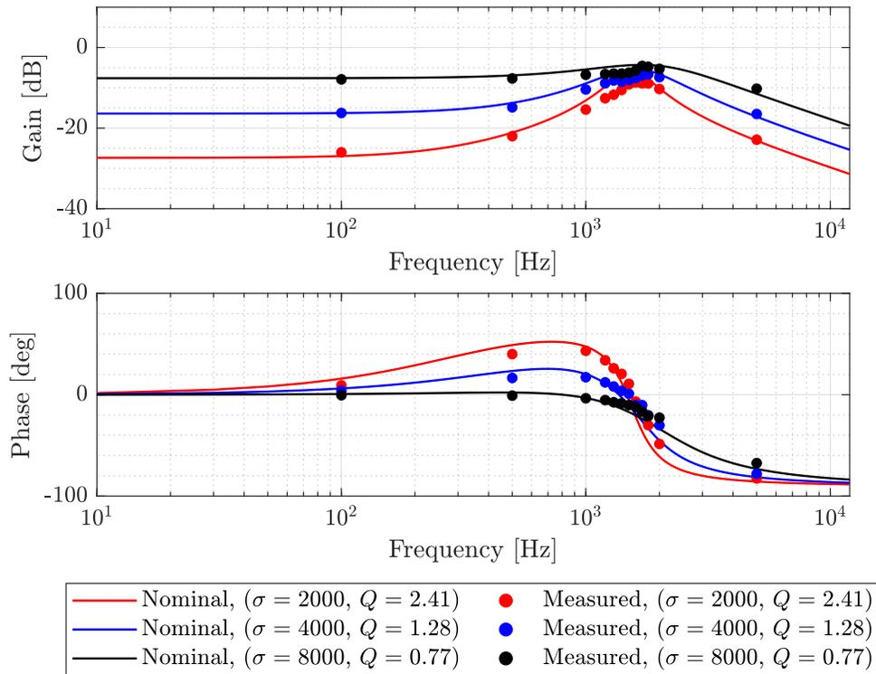
Figure 4.17: Comparison of measured frequency response in operating mode 2 of capacitor voltage  $v_{c,1}$  to perturbations in  $v_{c,1,ref}$  to the theoretical response  $\mathbf{H}_{CL,11}$  obtained from (4.47).
