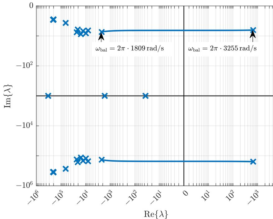
Figure 3.24: Eigenloci of the closed-loop small-signal generalized averaged model for a 6-level converter as the designed balancing loop bandwidth  $\omega_{\text{bal}}$  is varied. The model is derived with  $n = 5$  for the same design and operating conditions as the experimental measurement of Fig. 3.23, and verifies that  $\omega_{\text{bal}} = 2\pi \cdot 3255$  rad/s corresponds to an unstable design.
