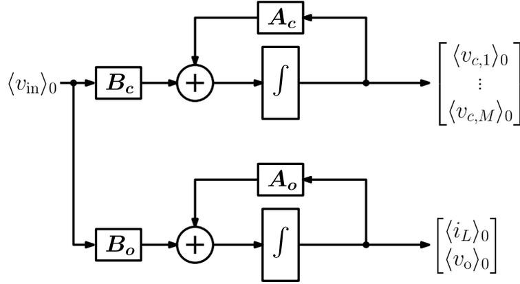
Figure 3.6: Block diagram representation of reduced-order model, showing the decoupled capacitor voltage and output filter dynamics.
