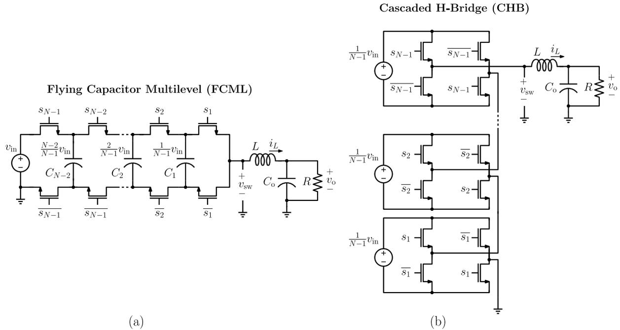
Figure 1.1: Two multilevel converters ((a) Flying Capacitor Multilevel (FCML) Converter; (b) Cascaded H-Bridge (CHB) Converter) exhibiting the properties studied in this introductory section.
