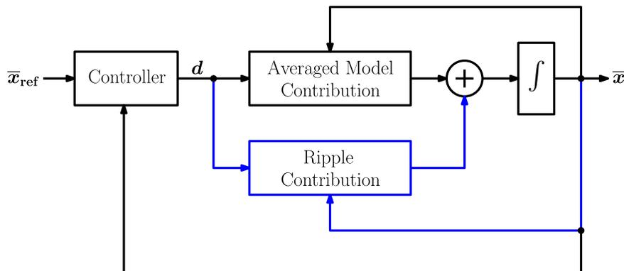
Figure 2.19: Representation of averaged dynamics used as the plant model in this chapter and faster unmodeled dynamics. The unmodeled ripple contribution is insignificant at moderate to heavy loads, but becomes more relevant at light loads, contributing to closed-loop instability depending on the choice of active balancing controller gains.
