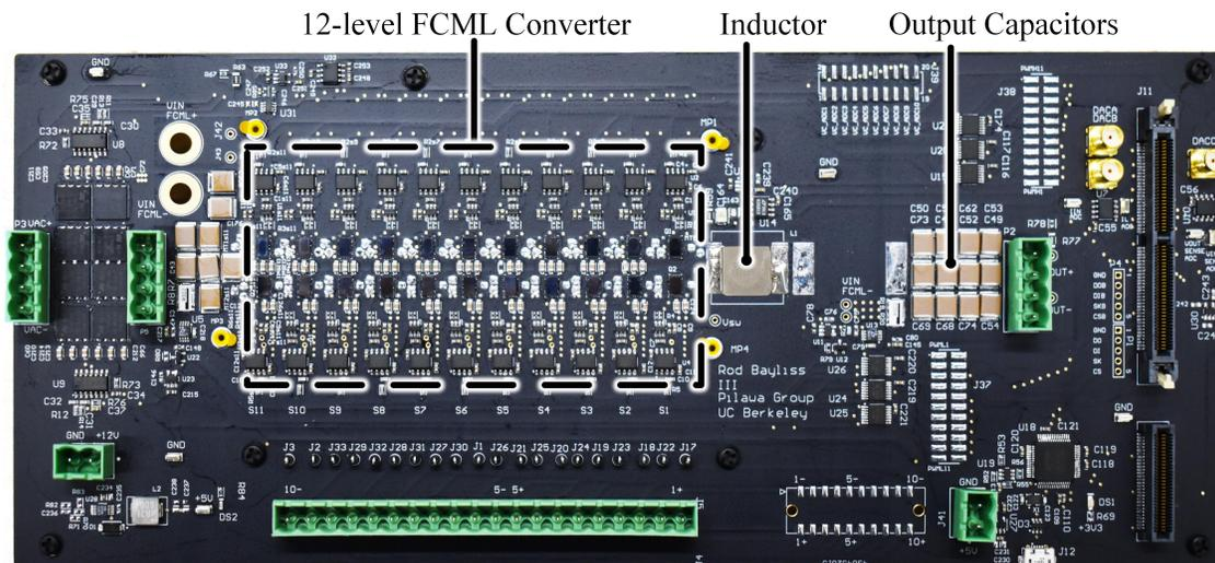
Figure 2.10: 12-Level FCML converter prototype with  $L = 10 \mu\text{H}$ ,  $C_k = 8.8 \mu\text{F}$ ,  $f_s = 100 \text{ kHz}$ . The parallel controller is implemented on a Texas Instruments TMS320F28379D DSP. The hardware is reconfigured as a 6-level FCML converter by shorting input-side switch pairs.
