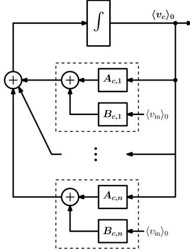
Figure A.2: Block diagram depiction of equivalent system when the feedback dynamic blocks in the full generalized averaged model represented in Fig. 3.3 are substituted with their dc gains. This structure is identical to the parallel feedback form shown in Fig. 3.9.
