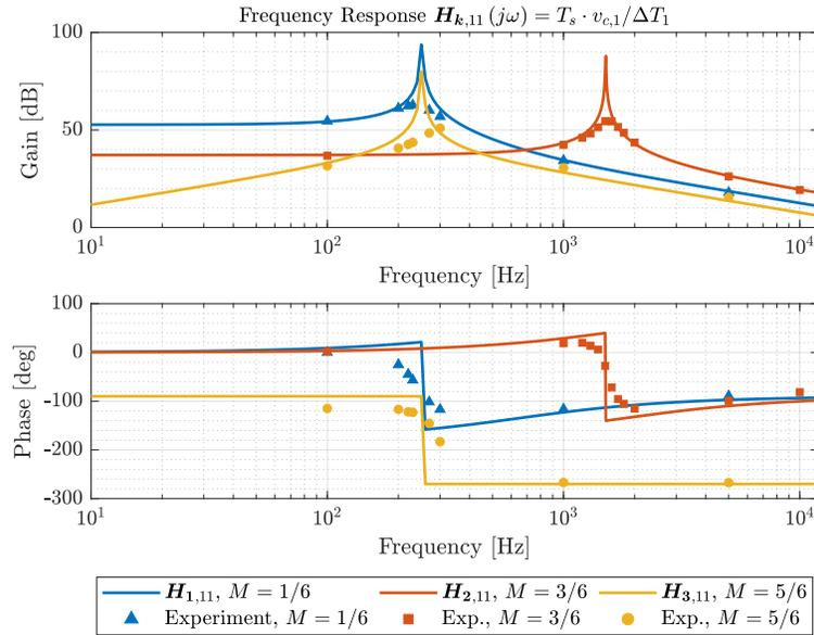
Figure 4.15: Comparison of measured frequency response of capacitor voltage  $v_{c,1}$  to perturbations in  $\Delta T_1$  to the theoretical response  $\mathbf{H}_{k,11}$  obtained from (4.34). The experimental measurements confirm the theoretical plant behavior in all operating modes, and exhibit nonzero damping arising from unmodeled parasitic elements in the converter.
