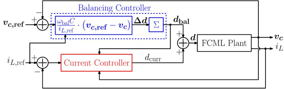
Figure 3.16: Parallel active balancing control structure detailed in Chapter 2.
