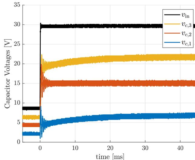
Figure 1.12: Measured voltage response in a 5-level FCML converter for a step in the input voltage  $v_{in}$  from 7 V to 30 V. The converter is configured with  $C = 8.8 \mu\text{F}$ ,  $L = 10 \mu\text{H}$ ,  $f_s = 75 \text{ kHz}$ , and  $R = 8 \Omega$ . Over a timescale of approximately 30 ms, the capacitor voltages balance to their respective nominal fractions of the input voltage.
