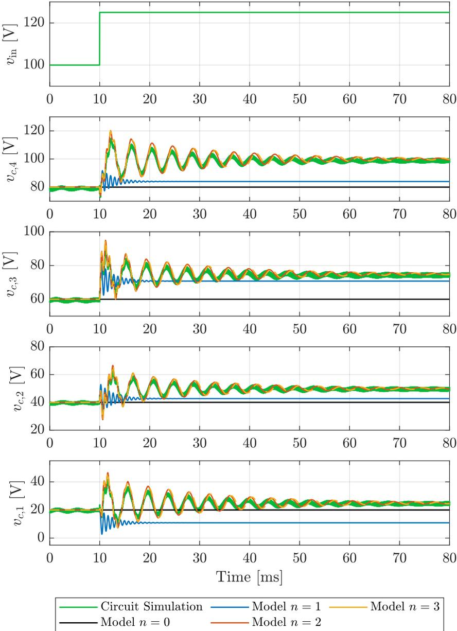
Figure 3.4: Simulated and modeled capacitor voltage responses for a 6-level FCML converter operating at  $D = 0.35$ , varying the total numbers of harmonics modeled  $n$ . The model with  $n = 2$  accurately captures the step-transient response. In the circuit simulation and model,  $L = 10 \mu\text{H}$ ,  $C = 8.8 \mu\text{F}$ ,  $R = 3.5 \Omega$ ,  $R_s = 0.3 \Omega$ , and  $f_s = 100 \text{ kHz}$ . The line voltage is stepped from 100 V to 125 V.
