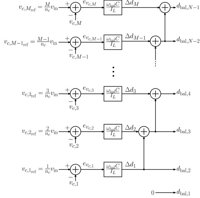
Figure 2.6: Block diagram representation of the balancing controller given in (2.42).
