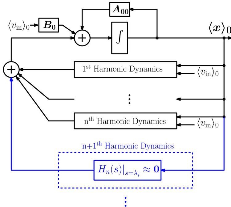
Figure 3.11: A Selective Modal Analysis (SMA) [123, 124, 126, 127] perspective on the  $n$ -term approximation of the generalized averaged model. The contribution of harmonics of order  $n + 1, n + 2, \dots, \infty$  to the  $p$  dominant modes studied are assumed to be zero.
