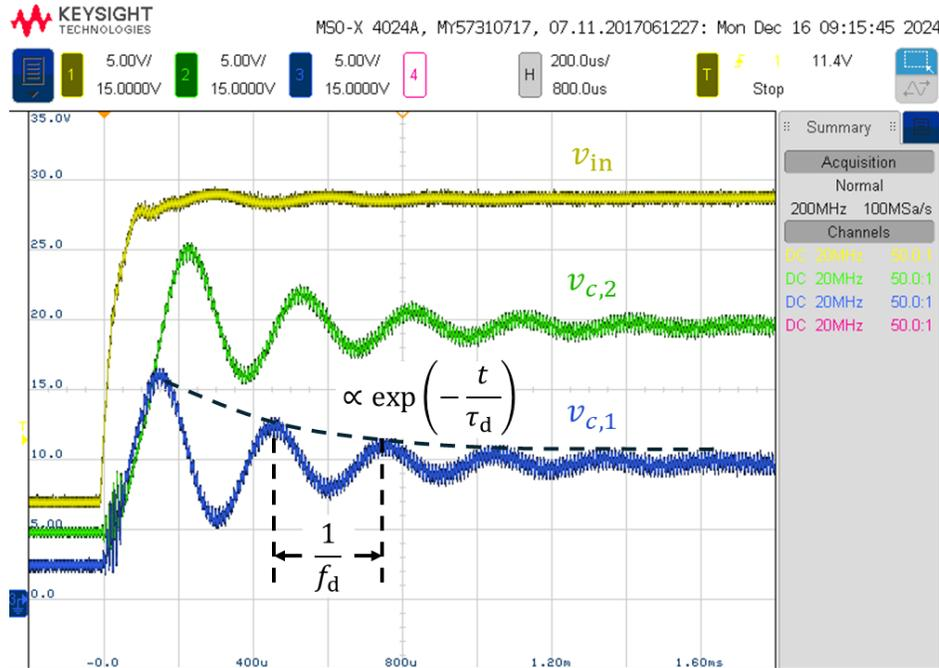
Figure 3.20: Measured response of capacitor voltages in a 4-level FCML converter operating at  $D = 0.5$  to a step in the input voltage from 7 V to 30 V. The measured responses are curve-fit to the general form of an exponential response to determine the time constant  $\tau_d$  and oscillation frequency  $f_d$  of the dominant mode. The converter tested has  $L = 4.7 \mu\text{H}$ ,  $C = 8.8 \mu\text{F}$ ,  $f_s = 100 \text{ kHz}$ .
