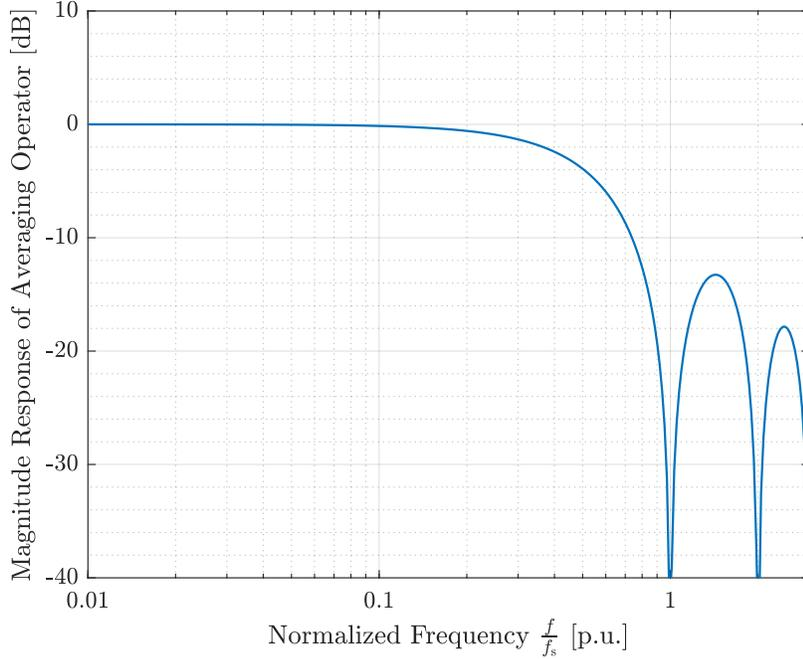
Figure 2.2: Magnitude response of averaging operator (2.4). Assuming the modulation frequency is significantly lower than the switching frequency ( $f_m \ll f_s$ ) the averaging operator captures the baseband content shown in Fig. 2.1.
