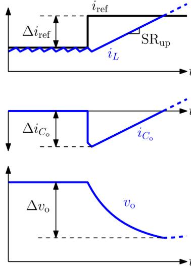
Figure 1.8: Illustration of the inductor current  $i_L$ , output capacitor current  $i_{C_o}$  and output voltage  $v_o$  during a transient in the inductor current reference  $i_{\text{ref}}$ . This scenario corresponds to the minimum output voltage deviation  $\Delta v_o$  during the load step-up transient.
