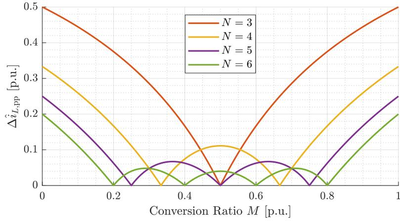
Figure 1.5: Normalized current ripple given by (1.9) plotted as a function of conversion ratio  $M$  for different level counts  $N = 3, \dots, 6$ .
