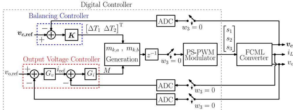
Figure 4.13: Block diagram representation of a single-sampled digital control architecture where the state-feedback balancing controller is implemented in parallel with a dual-loop output voltage controller.
