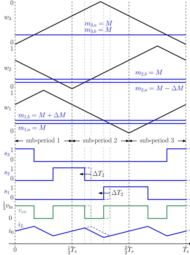
Figure 4.8: Carriers, modulating waveforms, and key converter waveforms for a 4-level FCML converter operating in mode 1 with a perturbation applied in sub-period 2. In the proposed implementation, two modulating waveforms  $m_{k,a}$  and  $m_{k,b}$  are associated with each triangular carrier  $w_k$ , and are used for up-count and down-count comparisons respectively.
