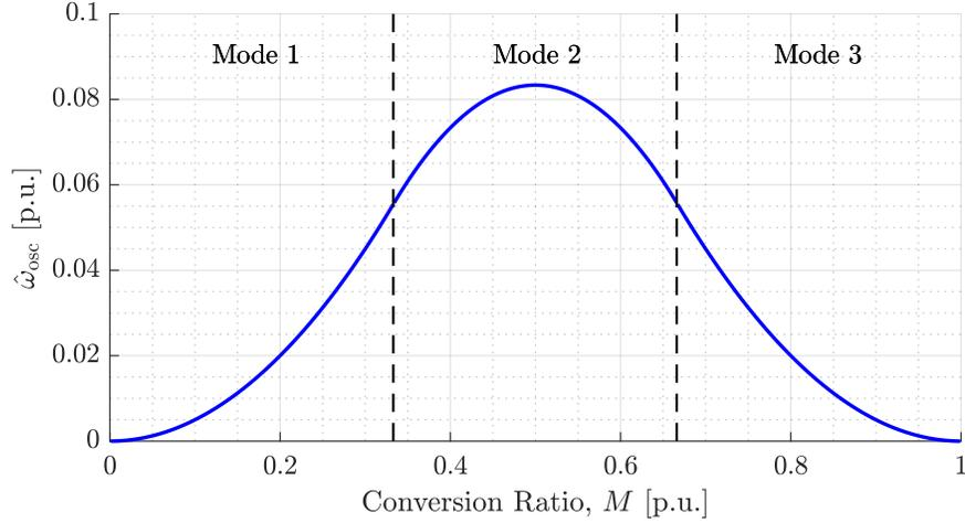
Figure 4.5: Normalized characteristic oscillation frequency  $\hat{\omega}_{\text{osc}}$  defined in (4.32) as a function of the conversion ratio  $M$ .
