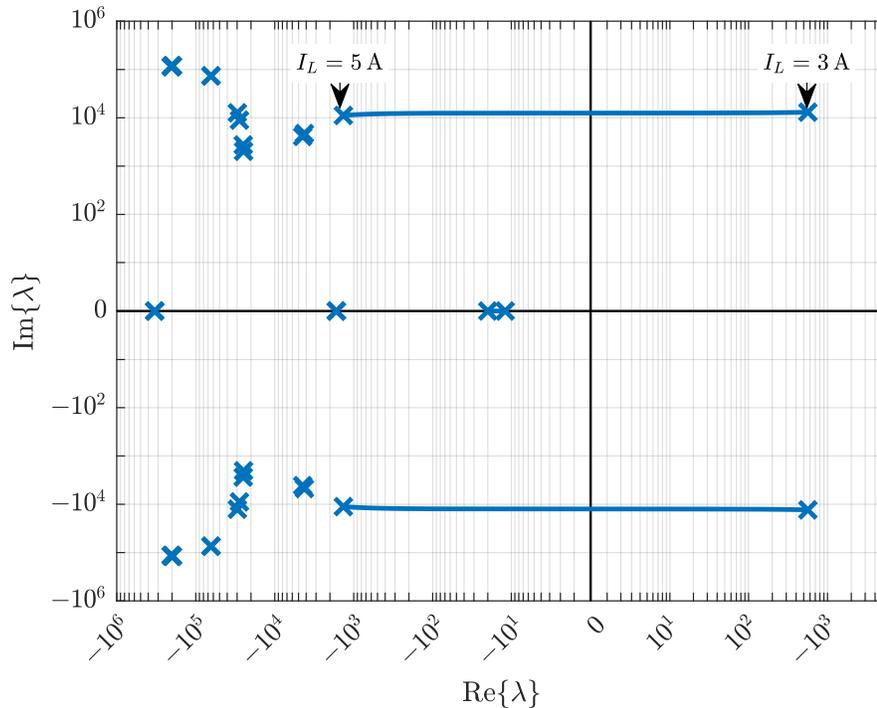
Figure 3.19: Eigenloci of the closed-loop small-signal model derived from generalized averaging as the average load current is varied. The model predicts the same instability observed in the simulation result of Fig. 3.18, with a relative error of 8% in the predicted oscillation frequency. The model is evaluated with  $v_{in} = 250$  V,  $D = 0.25$ ,  $L = 10$   $\mu$ H,  $C = 8.8$   $\mu$ F,  $R_s = 0.3$   $\Omega$ , and  $f_s = 100$  kHz.
