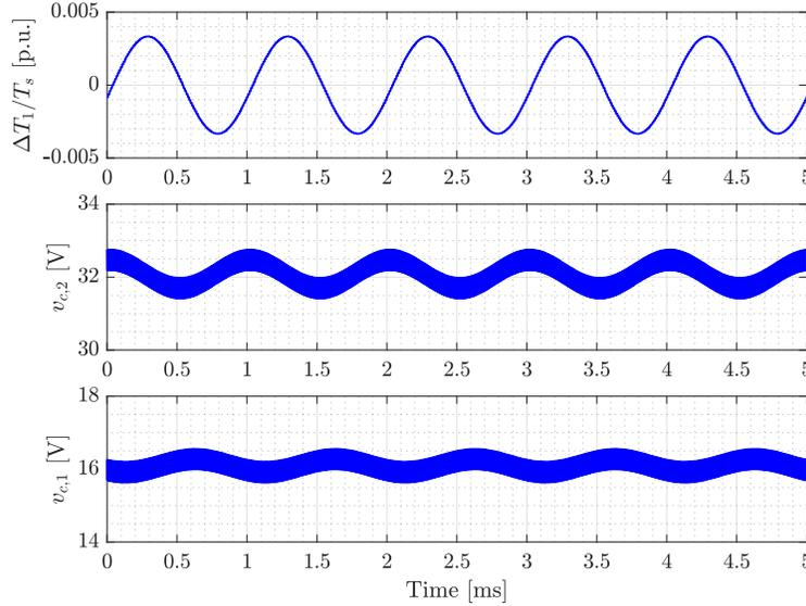
Figure 4.9: Simulated capacitor voltage responses for a 4-level FCML converter when applying a 1 kHz perturbation in control input  $\Delta T_1$ . The converter is operated with  $v_{in} = 48$  V,  $f_s = 100$  kHz,  $L = 10$   $\mu$ H, and  $C = 8.8$   $\mu$ F. The capacitor voltage responses are post-processed via Fast Fourier Transforms (FFTs) to determine the magnitude and phase response at the perturbation frequency.
