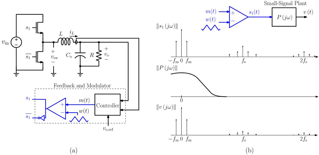
Figure 2.1: (a) General representation of feedback control and the pulse width modulator in a two-level converter; (b) Frequency domain representation of the open-loop small-signal system response to the pulse width modulated switching signal with modulation frequency  $f_m \ll f_s$ . Assuming the plant has a low-pass characteristic, the dominant components of the plant output  $v(t)$  occur at dc and the modulation frequency  $f_m$ .
