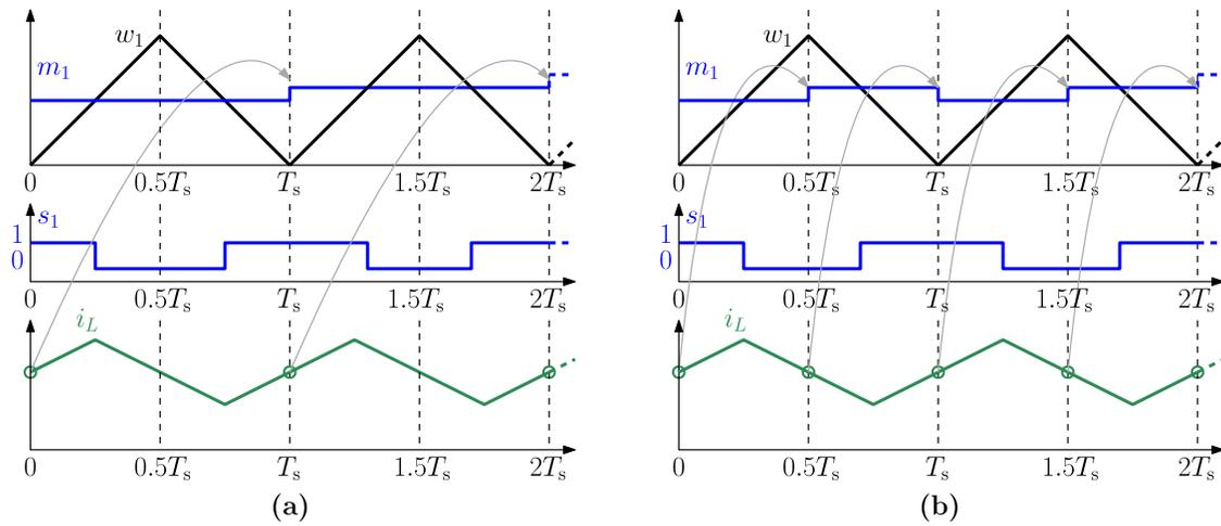
Figure 1.9: Digital PWM sampling and update modes for a two-level converter implementing average current control, considering a one-step computation delay: (a) single-sampling single-update at carrier valley; (b) double-sampling double-update at carrier peaks and valleys.
