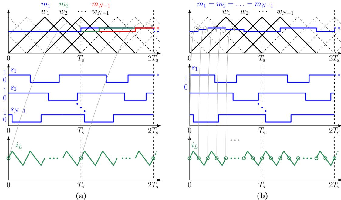
Figure 1.10: Digital PWM sampling and update modes for an  $N$ -level converter implementing average current control, considering a one-step computation delay: (a) single-sampling single-update at carrier  $w_1$  valley; (b) multi-sampling, multi-update at peaks, valleys, and intersections of all carriers [52]. For multilevel converters, double-update schemes are also possible, but are not shown in this figure for clarity.
