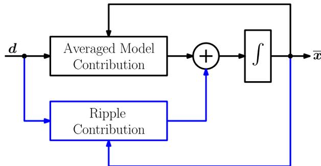
Figure 3.1: Block diagram representation of averaged plant model, showing the unmodeled impacts of the inductor current ripple.
