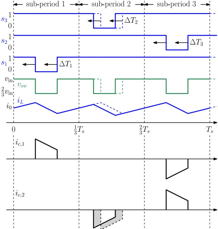
Figure 4.7: Converter waveforms illustrating the small-signal capacitor current response in operating mode 3 to a perturbation in the switching node voltage pulse position in sub-period 2. The small-signal impact of all perturbations is summarized in (4.26).
