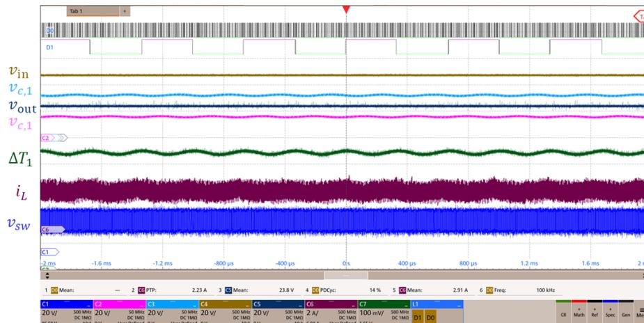
Figure 4.14: Oscilloscope waveform capture showing an example perturbation in  $\Delta T_1$  and measured capacitor voltages for the 4-level FCML converter prototype operating in mode 2. The data is post-processed using FFTs in MATLAB to determine the plant magnitude and phase response.
