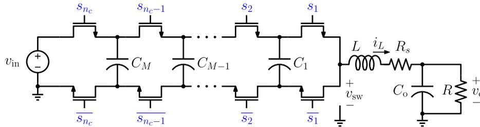
Figure 3.2: Schematic drawing of an  $N$ -level FCML converter, explicitly modeling a parasitic resistance  $R_s$ .
