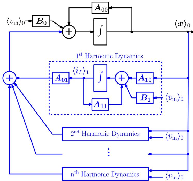
Figure 3.3: Block diagram of the full generalized averaged model given in (3.26). Contributions of the generalized averaged model compared to the standard averaged model are highlighted and appear as feedback dynamics.
