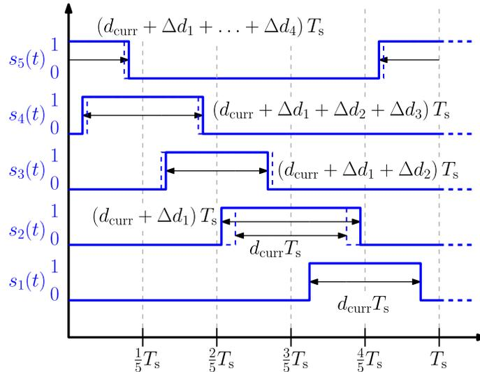
Figure 2.8: Example duty ratios applied to each switch resulting from simultaneous current control and active balancing actions. The balancing actions appear as difference duty ratios  $\Delta d_k$ , applied recursively to each switch beginning with  $d_1 = d_{curr}$ . The pulse width corresponding to the common-mode duty ratio  $d_{curr}$  is shown via dashed lines.
