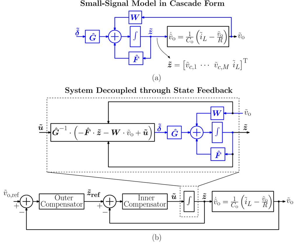
Figure 2.21: (a) Block diagram representation of the small-signal system in (2.21) in cascade form. (b) System resulting from the state feedback decoupling control law derived following the principles of [114]. This control law is identical to that presented in Section 2.3, but does not explicitly show the parallel control structure.
