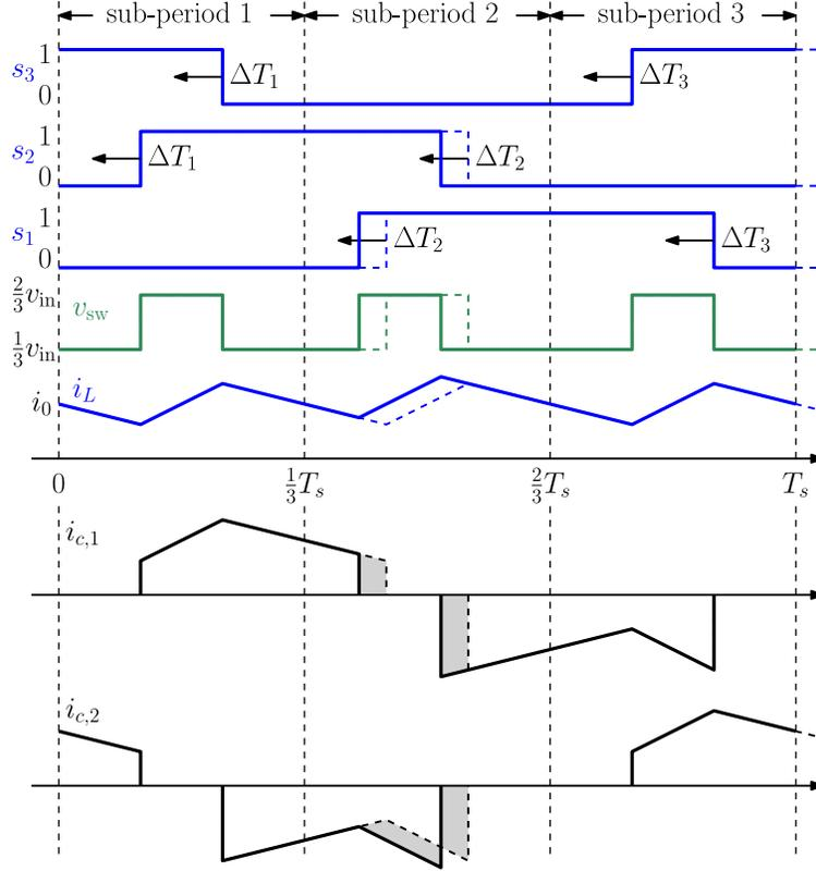
Figure 4.4: Converter waveforms illustrating the small-signal capacitor current response in operating mode 2 to a perturbation in the switching node voltage pulse position in sub-period 2. The differences in the quantity of charge flowing into each flying capacitor as a result of the perturbation are shown as shaded areas, and impact the capacitor voltages via the relations given in (4.8). The small-signal impact of all perturbations is summarized in (4.19).
