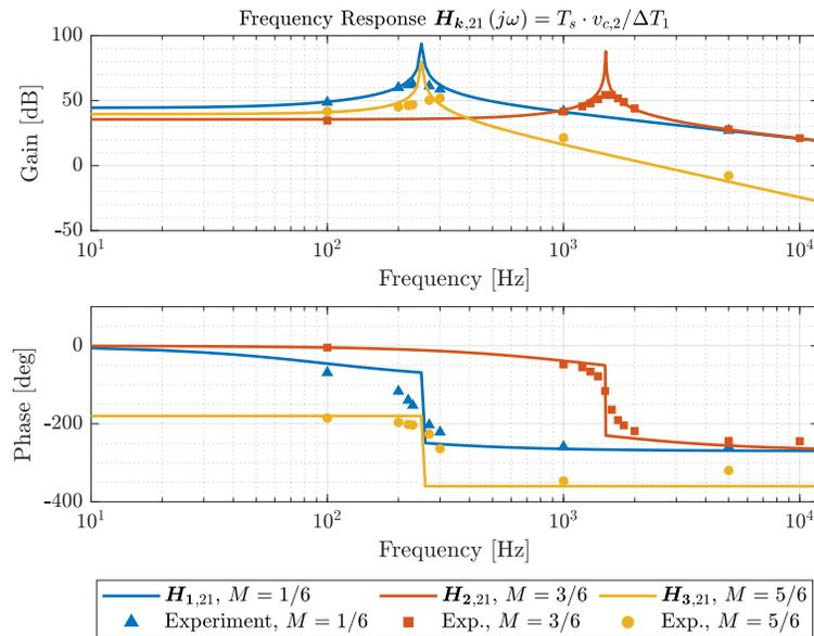
Figure 4.16: Comparison of measured frequency response of capacitor voltage  $v_{c,2}$  to perturbations in  $\Delta T_1$  to the theoretical response  $\mathbf{H}_{k,21}$  obtained from (4.34). The experimental measurements confirm the theoretical plant behavior, and exhibit nonzero damping arising from unmodeled parasitic elements in the converter.
