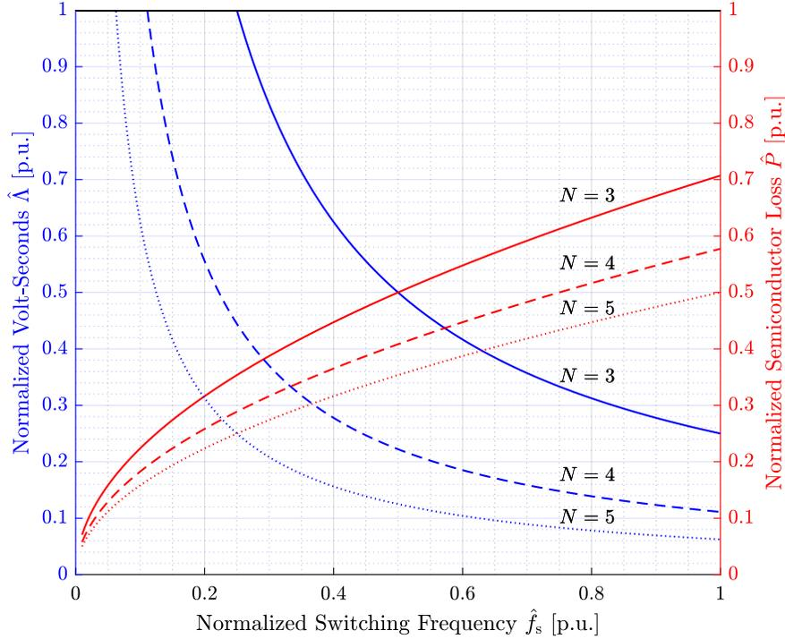
Figure 1.7: Normalized volt-seconds  $\hat{\Lambda}$  given by (1.11) and normalized semiconductor loss  $\hat{P}$  given by (1.17) plotted as a function of the normalized switching frequency  $\hat{f}_s$  defined in (1.18). An  $N$ -level converter performs better than a two-level converter in the range  $\frac{1}{(N-1)^2} < \hat{f}_s < 1$ .
