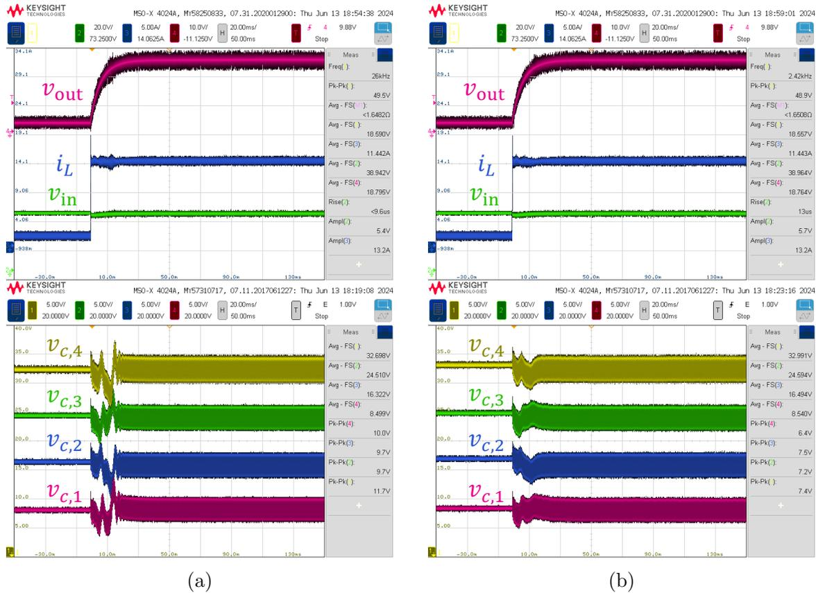
Figure 2.16: (a) Measured capacitor voltage response in the current-controlled converter relying on natural balancing during a large step change in the current reference from  $i_{ref}$  from 2 A to 15 A. (b) Measured capacitor voltage response in the current-controlled converter implementing the proposed active balancing controller. In both cases, the load transient is tested with  $v_{in} = 40\text{ V}$  and  $L = 4.7\ \mu\text{H}$ .
