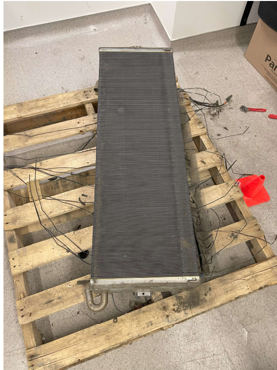
Figure 2.2: A photograph of a stack as extracted from the system of bus FC4. The horizontal lines through the stack represent the individual fuel cells while the pipe visible in the front of the stack shows the hydrogen input line. Pallet dimensions were approximately 5'x5'.
