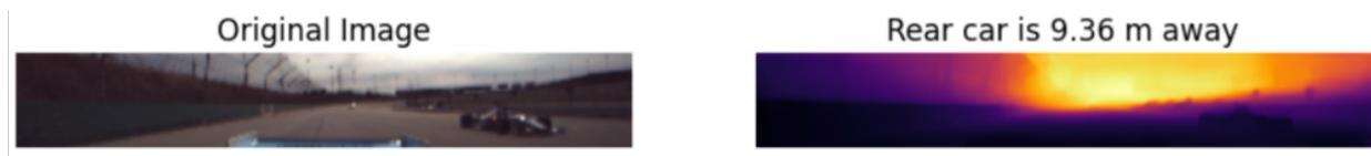
Figure 6.6: Output of depth estimation. Darker pixels are nearer.
