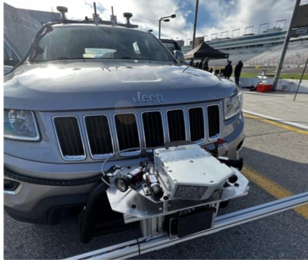
Figure 1.3: “Perception Jeep,” with front sensor mounting visible.
