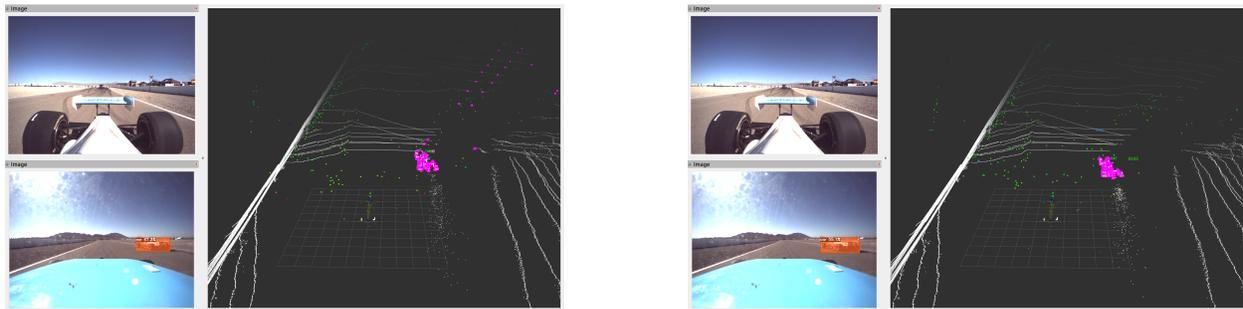
(a) Output of projection without binning. Note the presence of ground/wall points.
