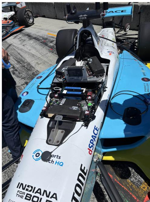
Figure 2.2: Autonomous electronics where the driver would usually sit.
