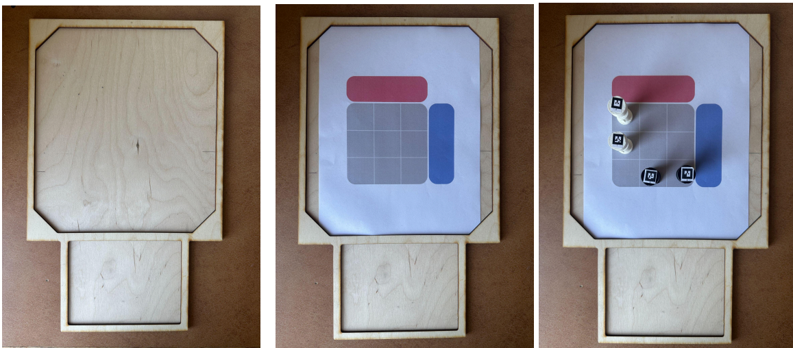
Figure 3.15: Custom wooden board – cutout for robot and paper game boards (left); printable SVG of Dodgem game board (middle); final setup with pieces on game board (right)
