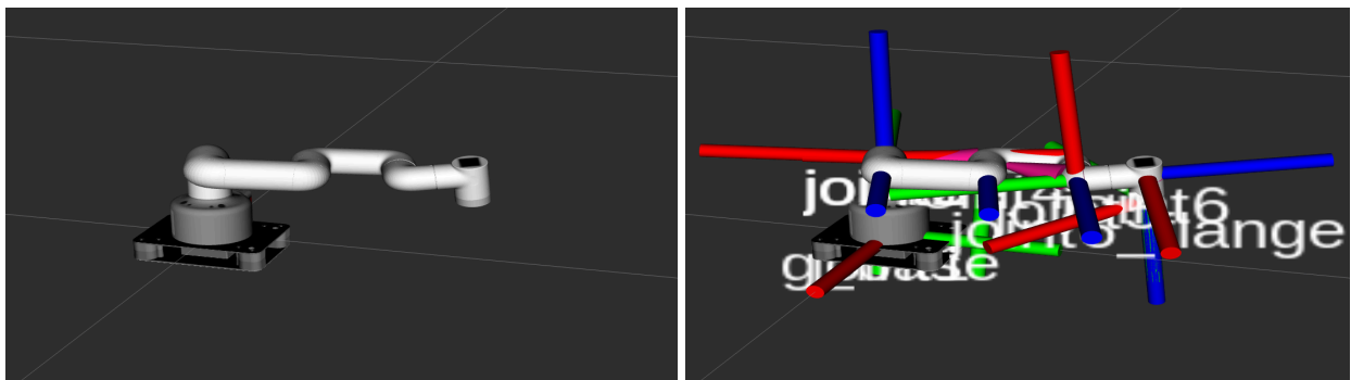
Figure 3.8: Full TF tree of MyCobot280pi in rviz – Before (left); After (right)
