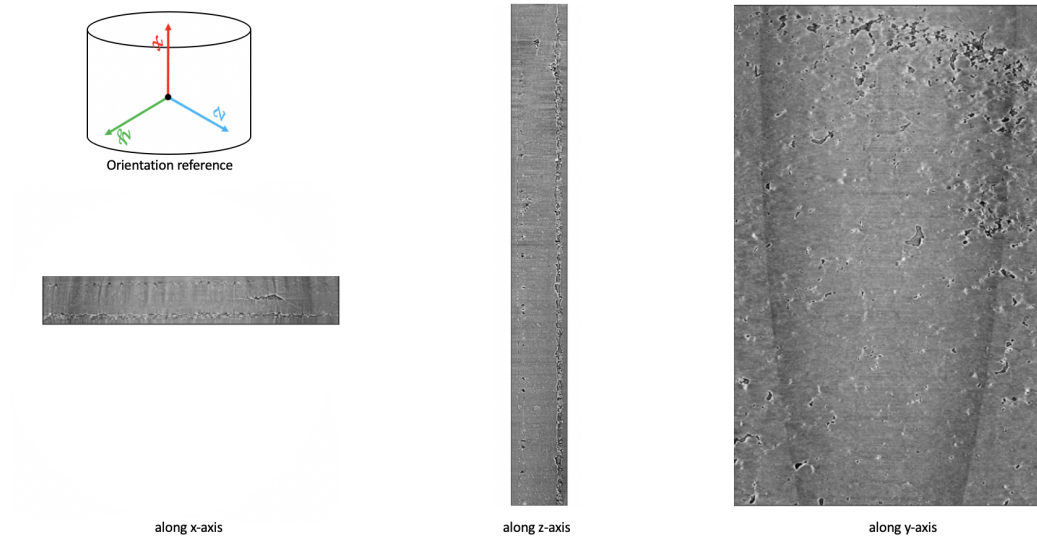
Figure 2.7: Sample Region of Interest (RoI) data obtained after pre-processing TomoPy reconstruction of a CT scan
