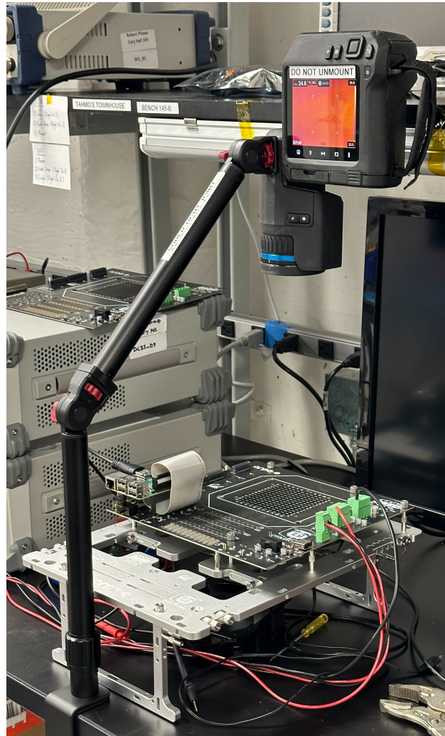
Figure 7.19: MCM TTV Demo for ARPA-E Energy Innovation Summit 2024. Includes a fully functional TTV operating in real-time with the thermal camera and GUI reporting the results.
