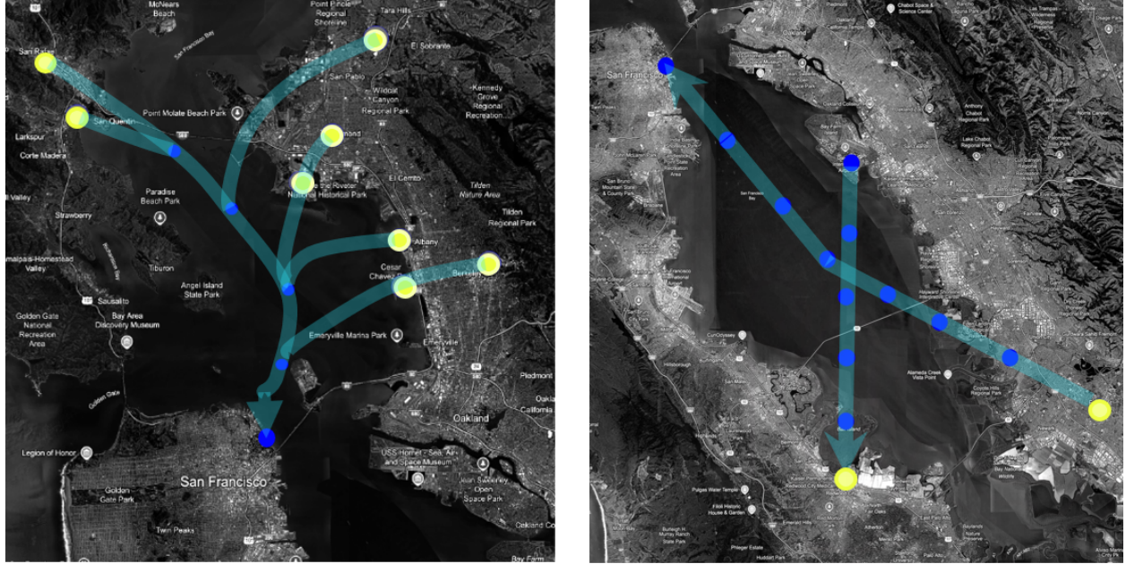
Figure 4.6: Bay Area case scenarios. The left panel illustrates routes where multiple air taxi vehicles would travel from the North and East Bay toward San Francisco, merging into a single air corridor. The right panel shows intersecting air corridors: one where the vehicles would travel from Fremont (southeast) to San Francisco, and another from Oakland (northeast) to Redwood City. The blue dots represent the waypoints that UAVs follow, while the yellow dots indicate the departure or an incoming waypoint of the corridor.
