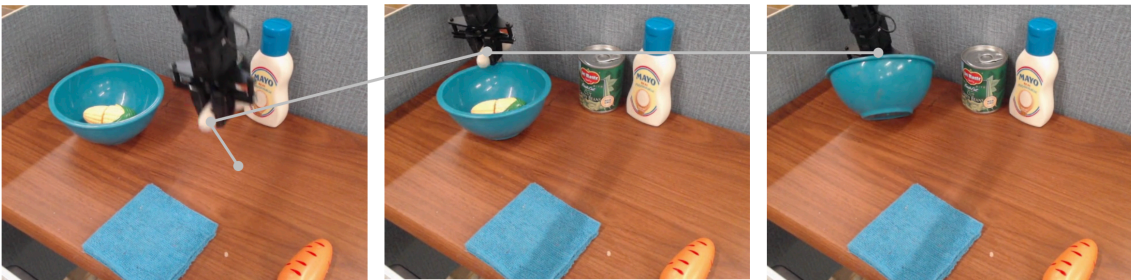
Figure 3.12: Grounding failure occurs when high level instruction is masked out. While the low level instruction “move the gripper left” correctly predicts the next reasonable action, masking out the context of the subtask “put the mushroom in the bowl” causes the policy to overshoot its trajectory.
