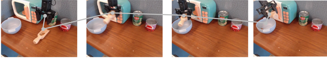
Figure 3.5: An execution of our method on the task “pour the contents of the scoop into the bowl.” Full breakdown of task and instructions can be seen at Section 3.4.
