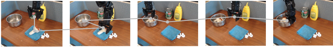
Figure 3.11: Spatial reasoning failure occurred when masking out low level instruction. The task was to “sweep the mints using the towel.” Due to the presence of the pot and the mushroom, being both strong priors within BridgeData, the policy chose not to follow the high level instruction.
