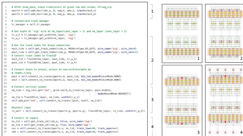
Figure B.1: Example inverter generator in BAG3.
