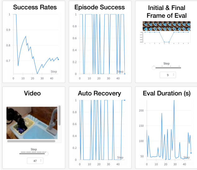
Figure 5: Excerpt from an AutoEval result report, provided to the user upon completion of the automated evaluation. Users can see the per-episode success rate, rate of evaluation progress, instances of automatic recovery from motor failures, and qualitative rollout videos as well as classifier result plotted with initial and final frames to obtain a wholistic understanding of the policy’s performance.
