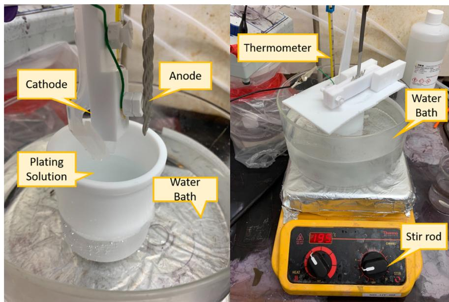
Fig. 2.15: All fixtures are custom-designed and fabricated from Teflon. The setup enables precise control of electroplating parameters, including the spacing between the cathode and anode, the depth of the sample in the plating solution, plating uniformity across samples or wafers, and other critical factors.
