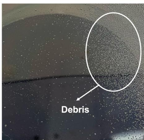
Fig. 2.11: The deposited a-Si film appears blurry and contains debris-like inclusions, highlighting cleanliness issues with the a-Si mold that need to be addressed.
