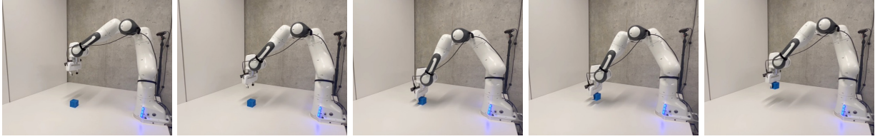
Figure 4.7: Real-world Deployment: We show an example episode of our policy performing the cube picking task on a Franka robot in the real world. We use Toto -base to run the robot at real time, despite being a small model, Toto was able to achieve about 63% success rate in real world setting.
