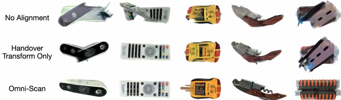
Figure 3.6: **Alignment Ablation** We perform an ablation on the alignment as illustrated in Fig. 3.3 on 5 objects. We present renders for models with no alignment, with only handover transform, and Omni-Scan which uses the handover transform as an initialization for ICP alignment.
