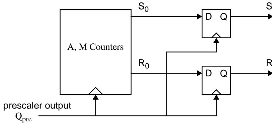
Fig. 5.13: Counter outputs re-clocking
