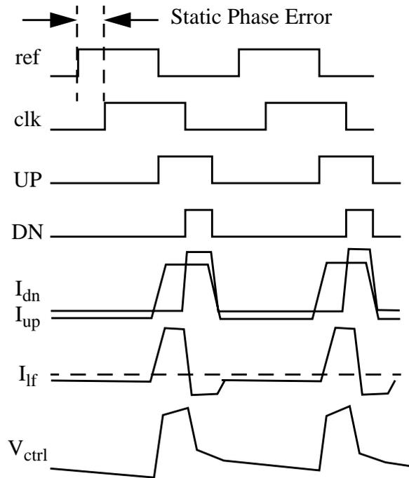
Fig. 4.18: Waveforms of the loop filter with nonidealities
