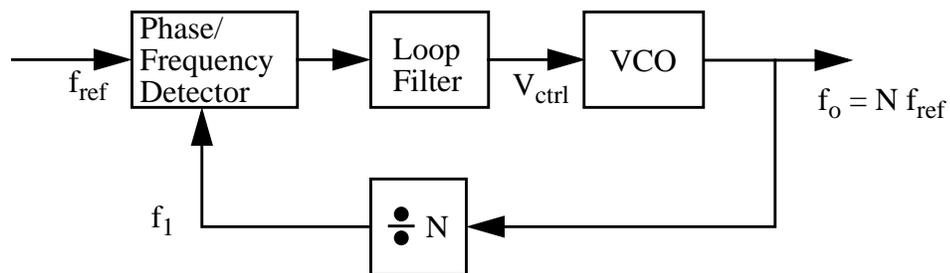
Fig. 2.6: Phase-Locked-Loop block diagram
