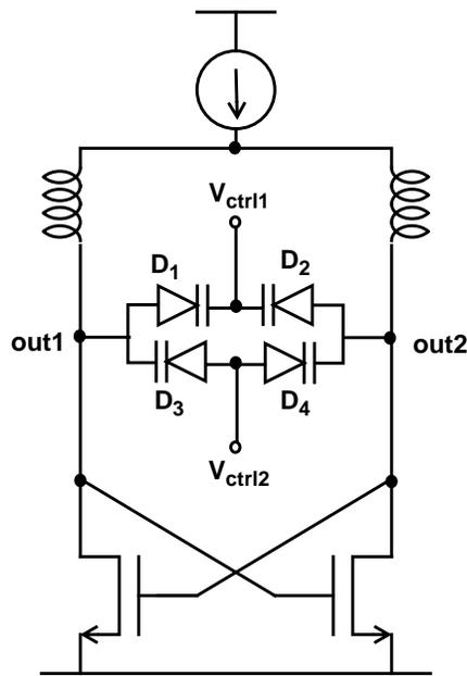
Fig. 4.15: Differentially-controlled VCO with differential output
