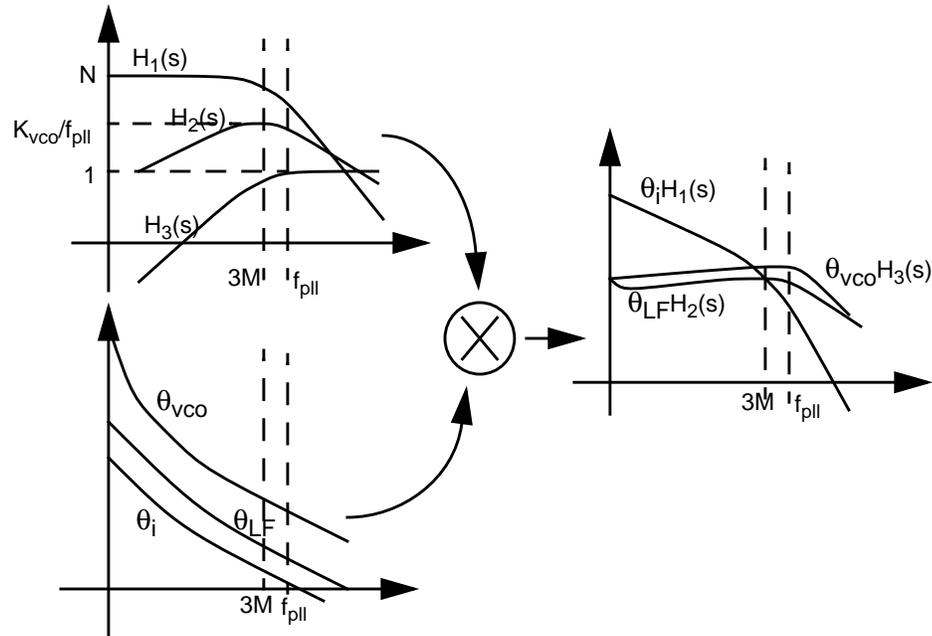
Fig. 3.4: Loop bandwidth optimization example for a second order PLL
