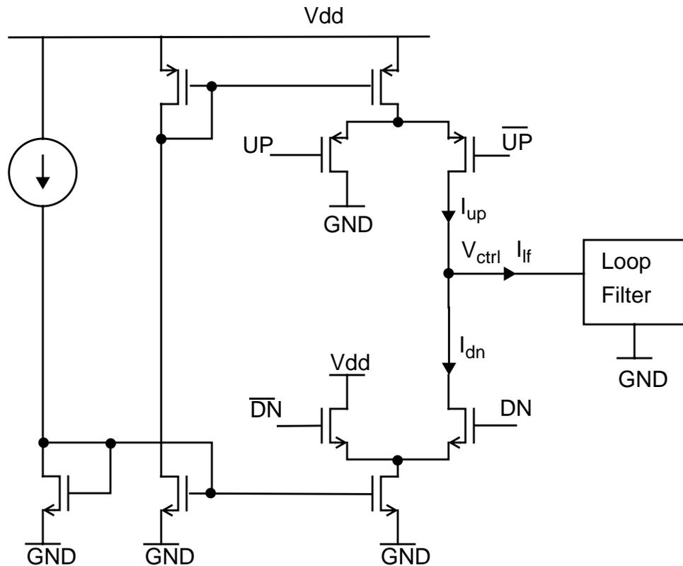
Fig. 4.17: Current steering charge pump
