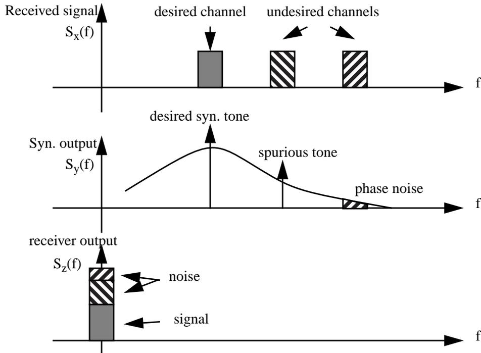
Fig. 5.3: Effect of phase noise and spurious tones in a receiver
