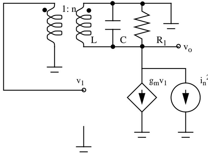
Fig. 4.13: Equivalent noise model
