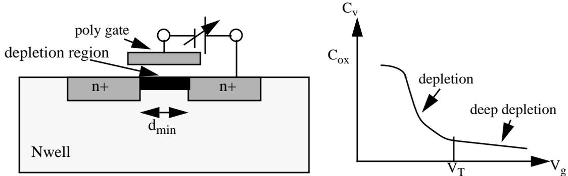
Fig. 4.9: Cross section of a MOS capacitor and its C-V curve
