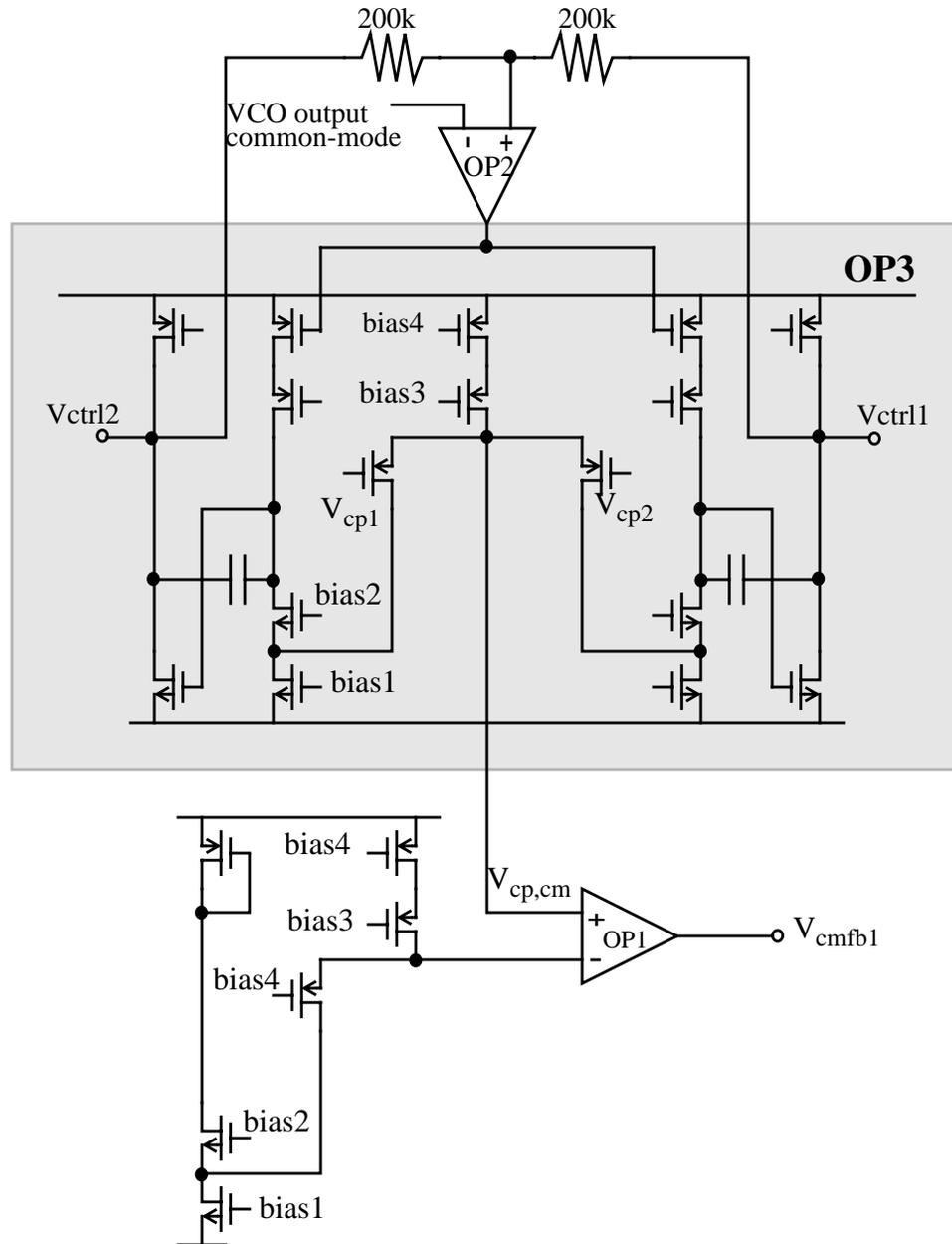
Fig. 5.11: Detailed circuit of OP3 and its input/output CMFB
