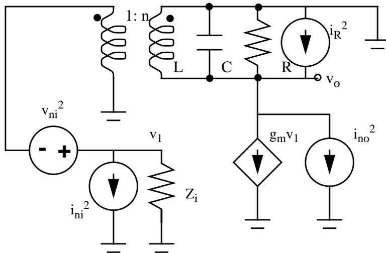
Fig. 4.12: Noise model of a basic positive feedback amplifier with loop gain  $< 1$
