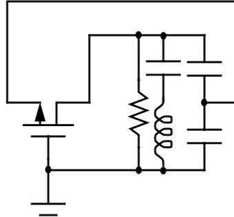
Fig. 4.11: Clapp oscillator
