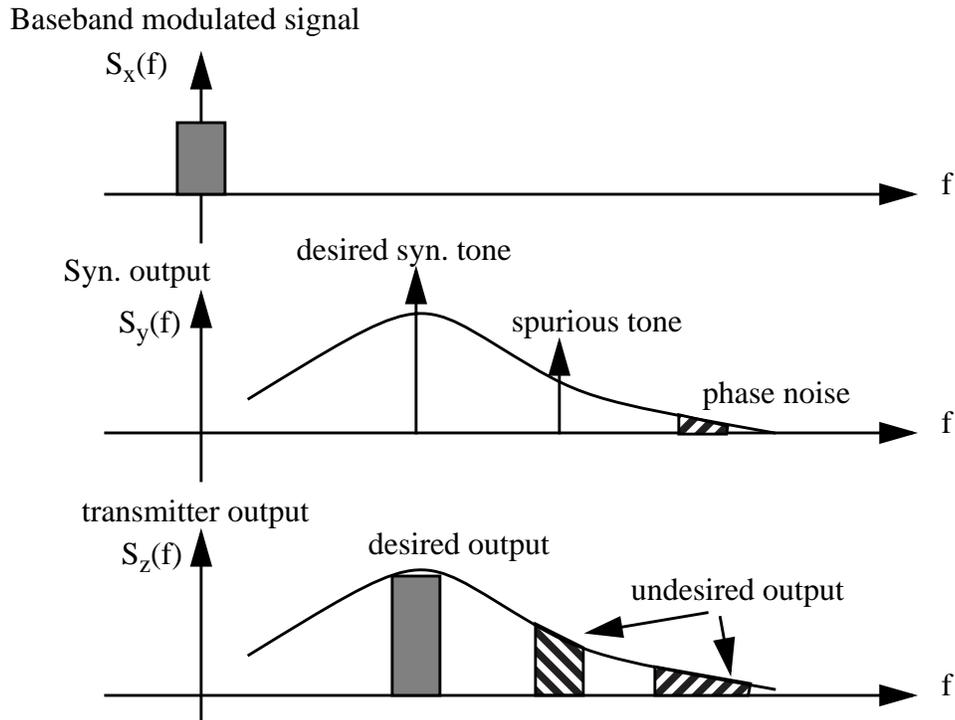
Fig. 2.4: Effect of phase noise and spurious tones in a transmitter
