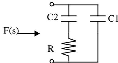
Fig. 5.7: Loop filter based on RC
