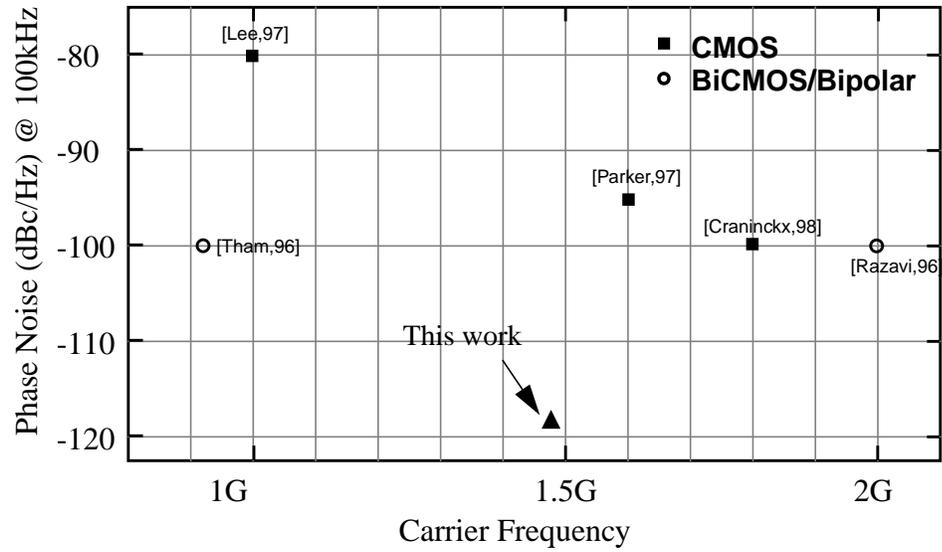
Fig. 5.21: Comparison of recently published work on integrated synthesizer
