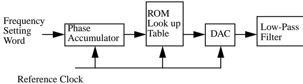
Fig. 2.5: DDFS block diagram
