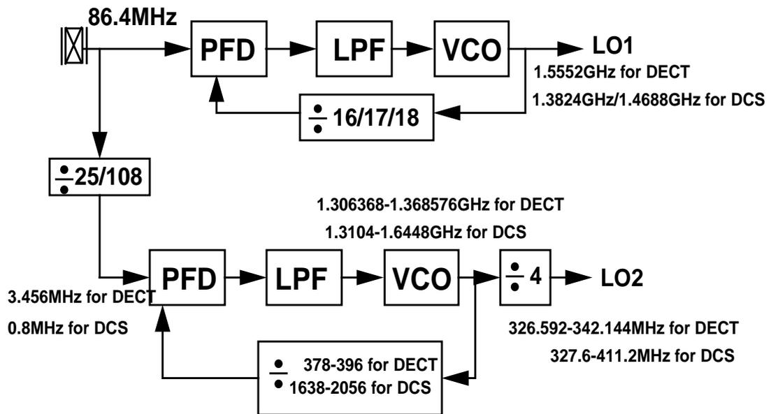
Fig. 5.6: PLL implementation of the frequency plan
