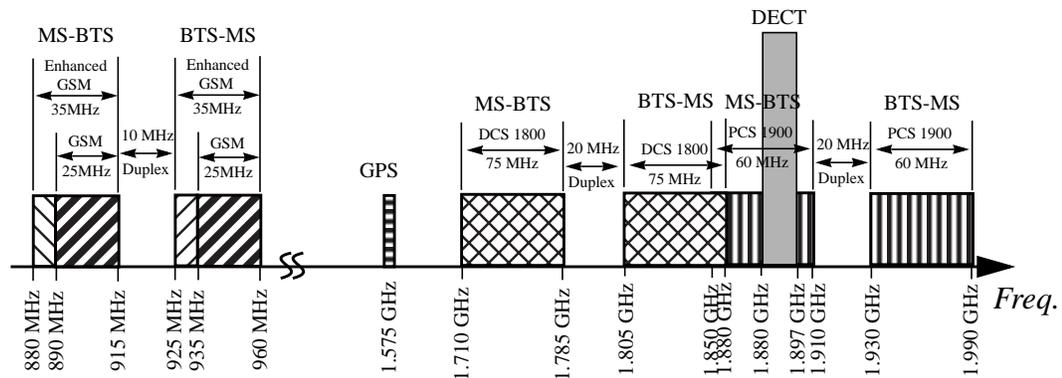
Fig. 5.1: Band allocation of various standards
