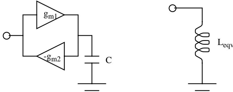
Fig. 4.6: On-chip active inductor
