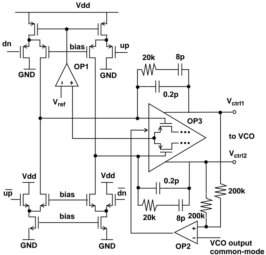
Fig. 5.10: Charge pump with active loop filter for LO1
