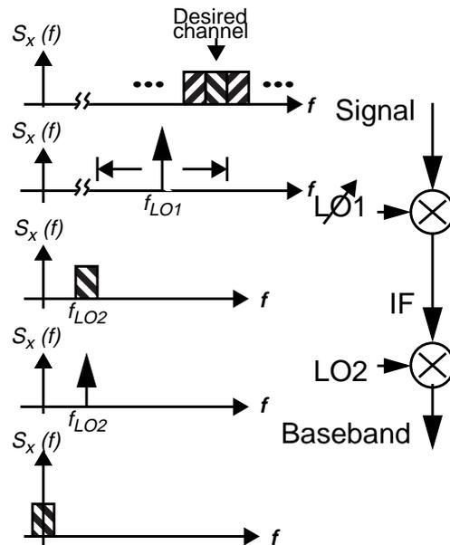
Fig. 3.5: Spectrum translation in Superheterodyne receiver architecture
