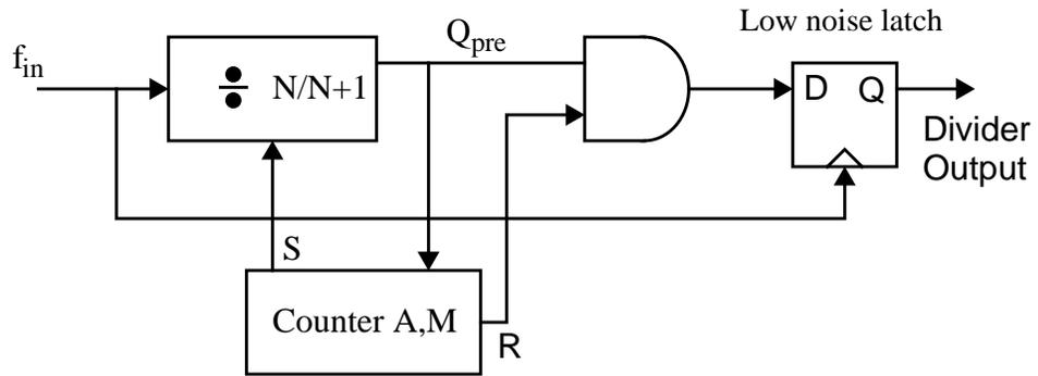
Fig. 5.12: Low noise latch input re-clocked by prescaler output
