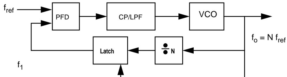
Fig. 5.5: PLL block diagram
