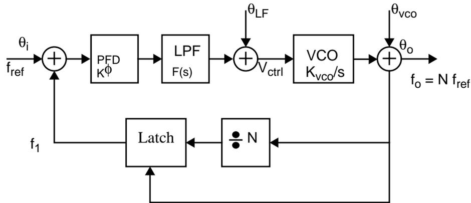
Fig. 4.1: PLL block diagram
