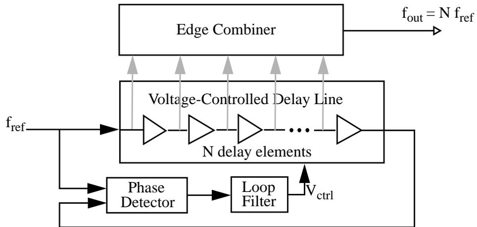
Fig. 2.9: Block diagram of a Delay-Locked Loop frequency synthesizer
