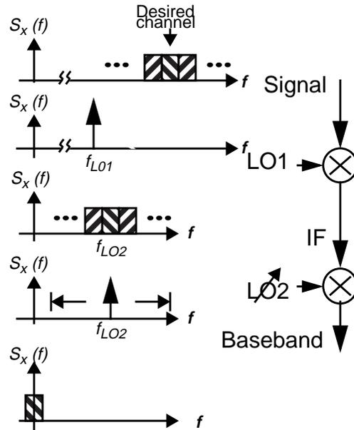
Fig. 3.6: Spectrum translation in the Wideband IF Double Conversion Receiver Architecture
