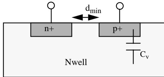
Fig. 4.7: Cross section of the p+/Nwell junction
