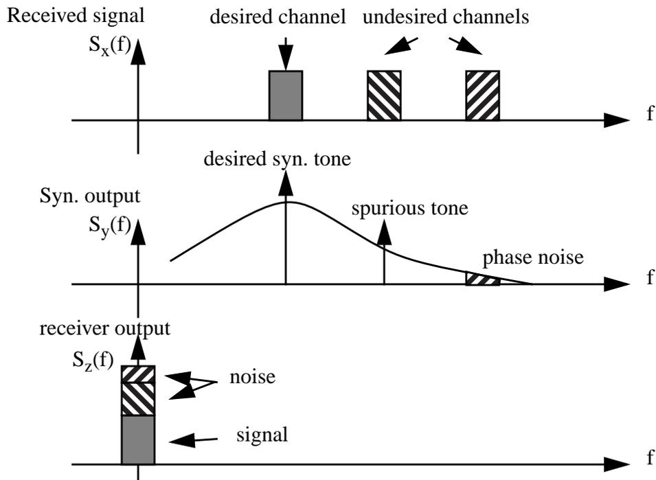
Fig. 2.3: Effect of phase noise and spurious tones in a receiver
