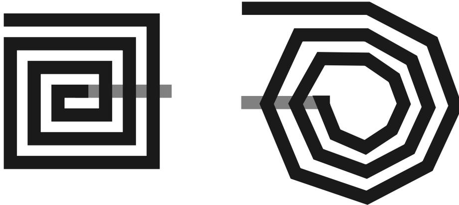
Fig. 4.4: Square and octagonal spiral inductors
