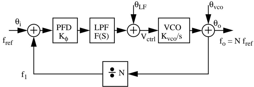
Fig. 2.7: Phase-Locked-Loop linear model
