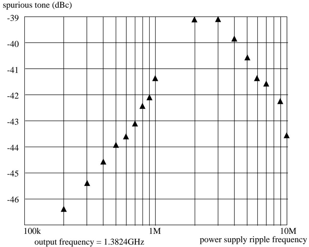
Fig. 5.20: Supply sensitivity vs. power supply ripple frequency
