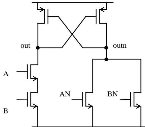
Fig. 4.23: Two input AND/NAND DCVSL gate
