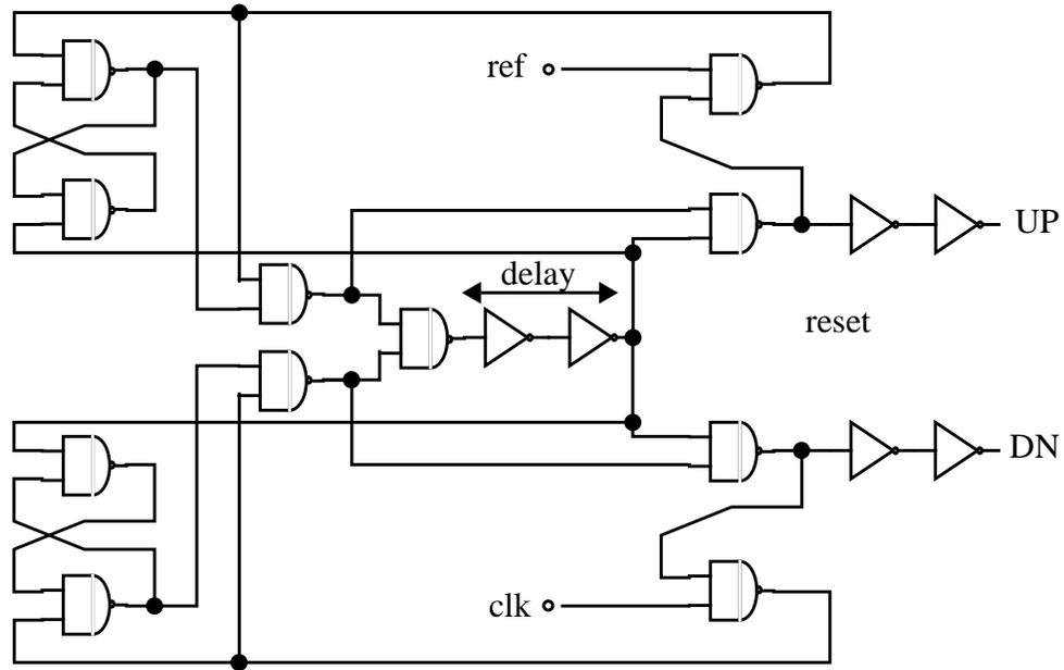
Fig. 4.22: Phase/frequency detector circuit diagram
