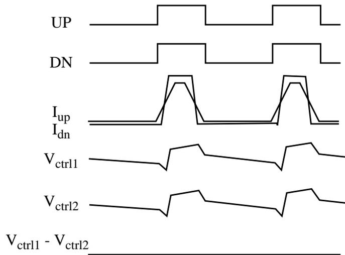
Fig. 4.20: Waveforms of differential charge pump with nonidealities
