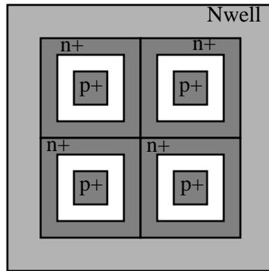
Fig. 4.8: An array of the varactor
