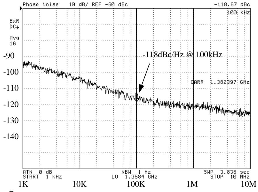
Fig. 5.18: Measured phase noise performance
