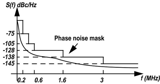
Fig. 5.4: Phase noise specifications for DCS1800
