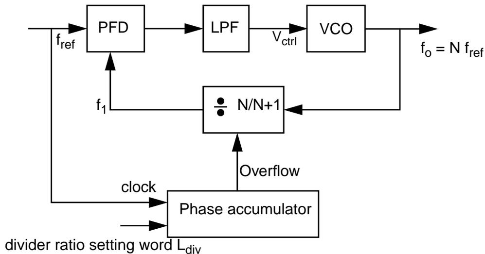
Fig. 2.8: Fractional N frequency synthesizer block diagram
