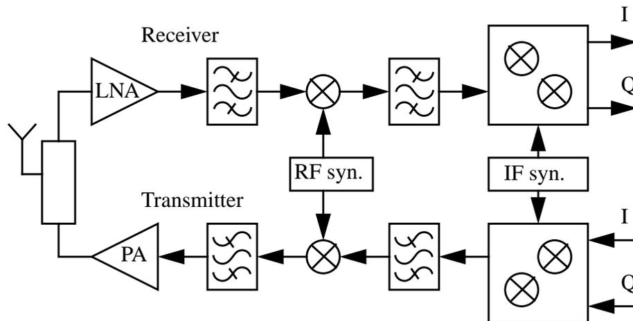
Fig. 2.1: Synthesizer in cellular application
