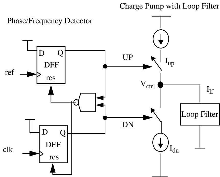
Fig. 4.16: Functional block diagram of the loop filter and PFD
