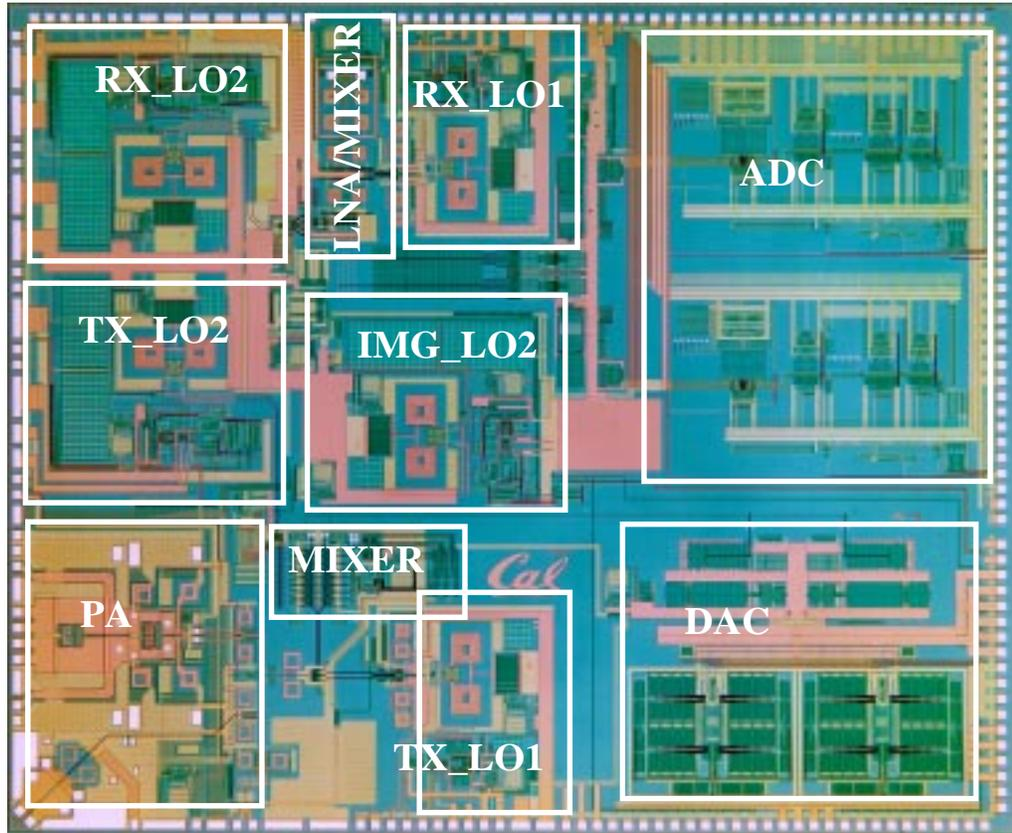
Fig. 5.17: Die Micrograph of complete transceiver including LO1 and LO2 for both transmitter and receiver
