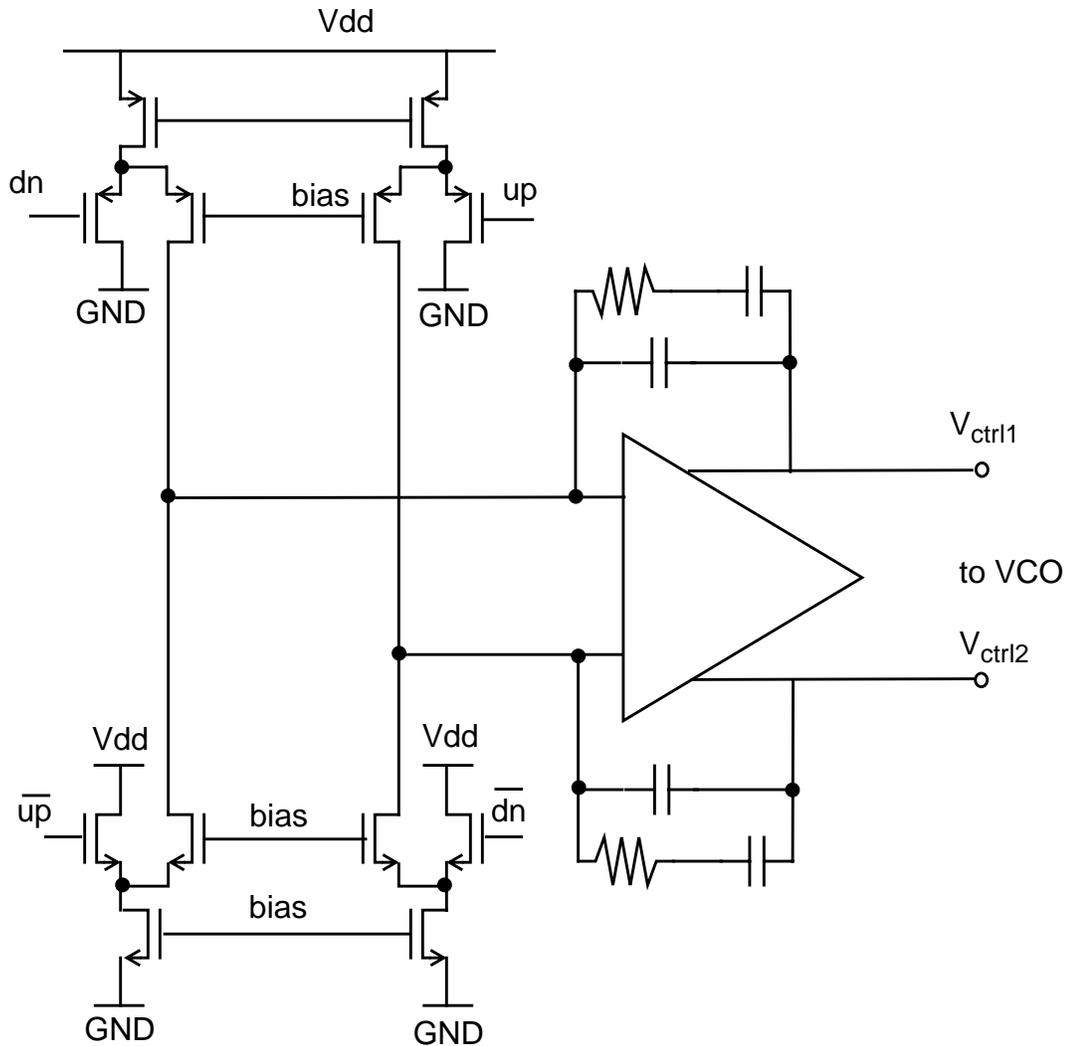
Fig. 4.21: Differential charge pump with active loop filter
