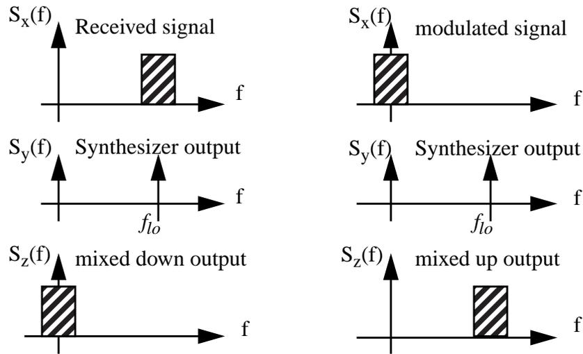
Fig. 2.2: Role of frequency synthesizer
