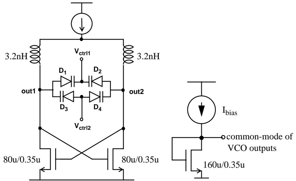
Fig. 5.8: Differentially controlled VCO with differential outputs
