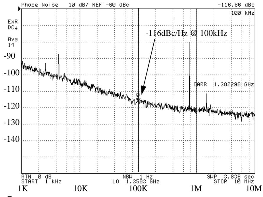
Fig. 5.19: Measured phase noise when a 100mv 0-to-peak sinewave at 0.8MHz is applied to power supply
