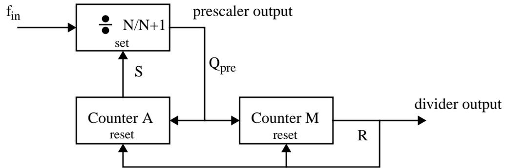
Fig. 4.25: Block diagram of a programmable divider
