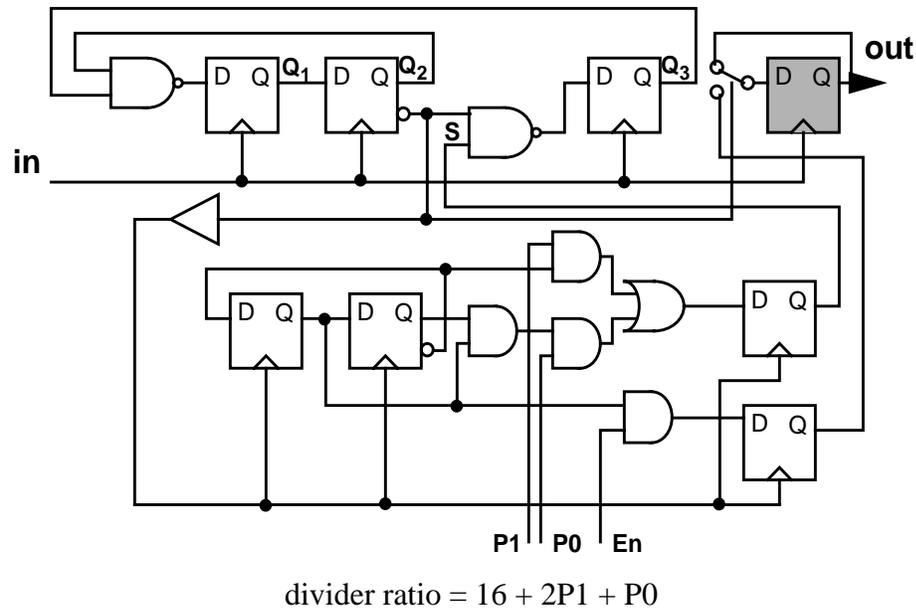
Fig. 5.14: Block diagram of a prescaler with dividing ratio 16/17/18
