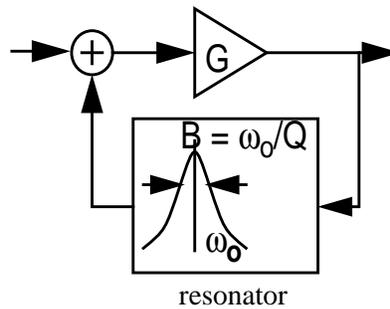
Fig. 4.3: Tuned oscillator model
