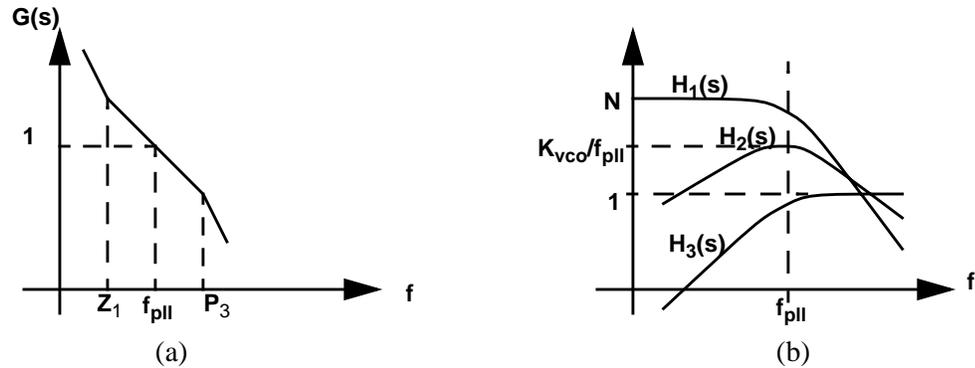
Fig. 3.2: Transfer functions of the 2nd-order PLL a) open-loop gain b) transfer functions
