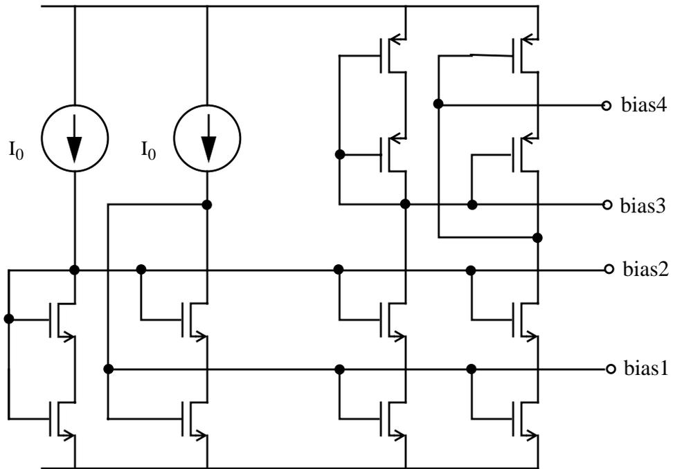
Fig. 5.9: Bias circuit for charge pump
