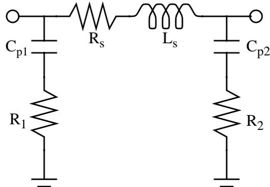
Fig. 4.5: Spiral inductor model
