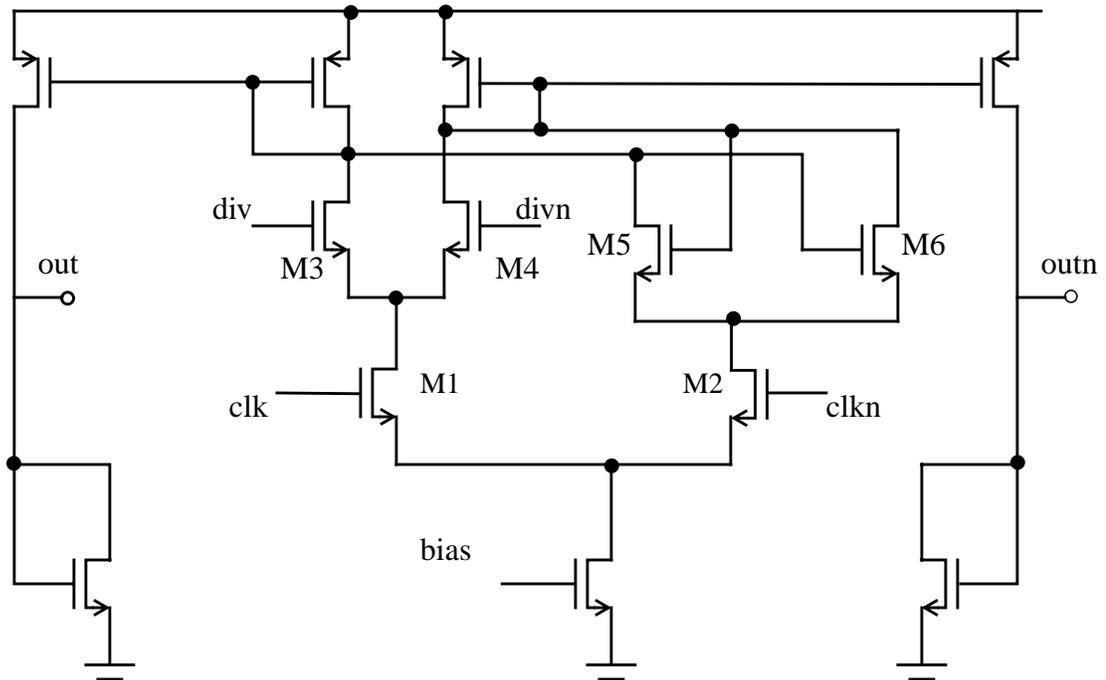
Fig. 4.24: Low-noise latch clocked by VCO
