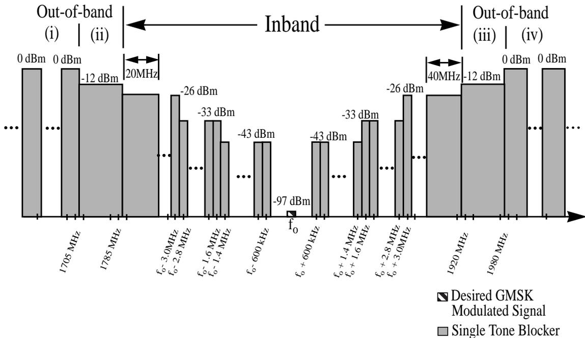
Fig. 5.2: Blocking characteristics of DCS1800
