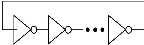
Fig. 4.2: Block diagram of a ring oscillator
