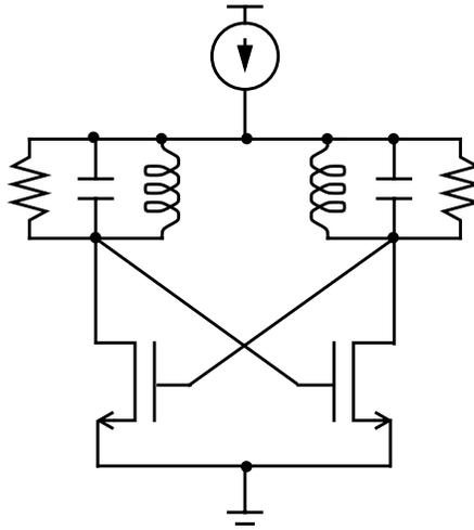
Fig. 4.14: Differential VCO with cross coupled pair
