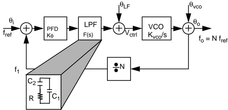
Fig. 3.1: Second Order Phase-Locked Loop linear model
