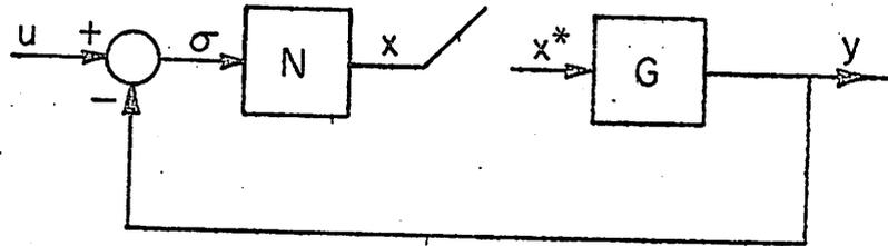
Fig. 1. Time-varying nonlinear sampled-data feedback system.
