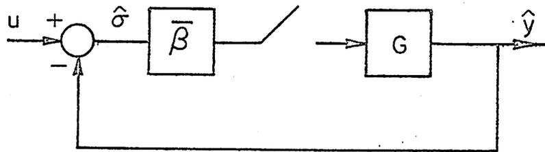
Fig. 2. Linearized sampled-data feedback system.
