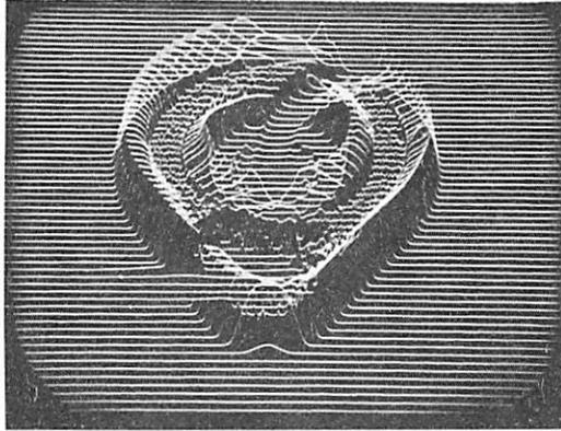
Fig. 1. Deflection-modulation display of an NPN transistor generated by electron-beam-induced currents. Scanning electron beam voltage = 15 kv; 64 line raster.
