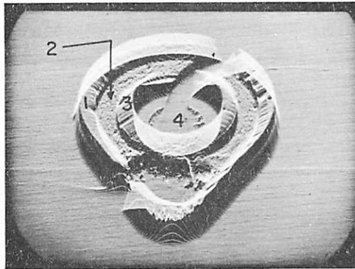
Fig. 2. Deflection-modulation display of same subject as Fig. 1; 64 line raster.
