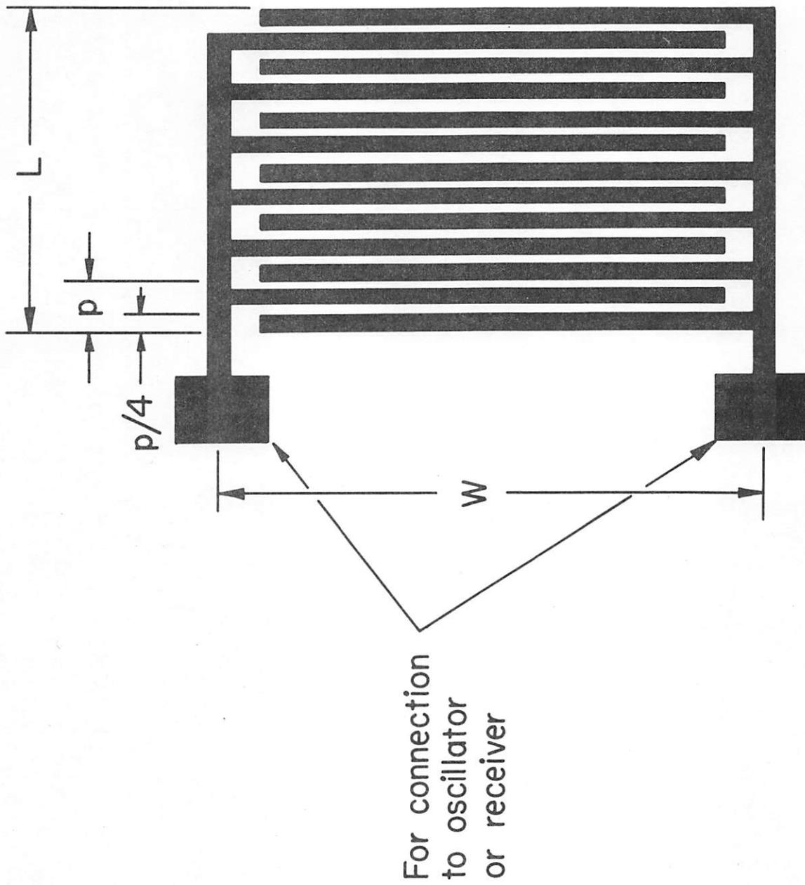
Fig. 1b. Electrode pattern used in (a) at 15 and 45 mc.
