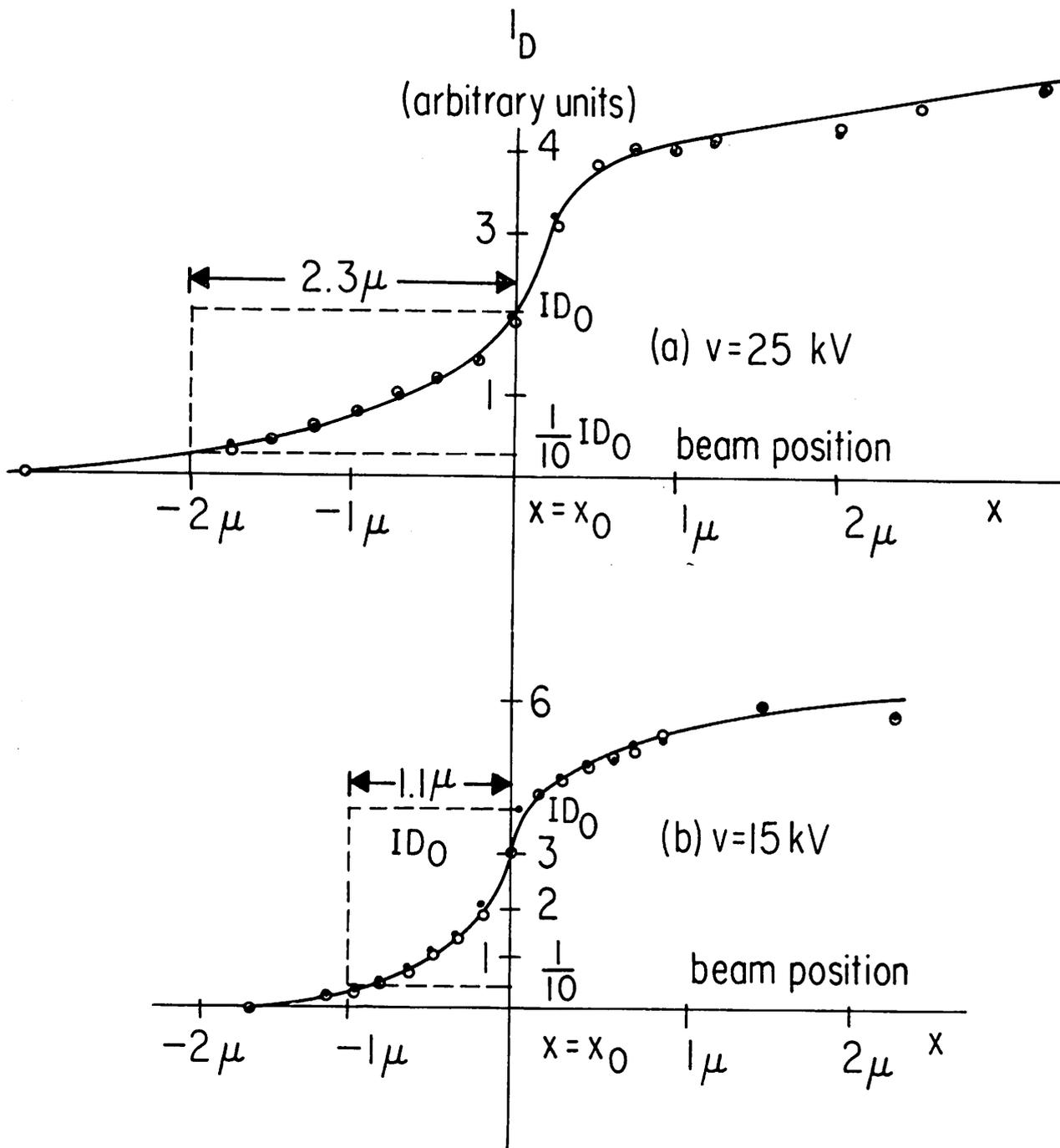
Fig. 2 Measurements of  $I_D$  as a function of beam position.
