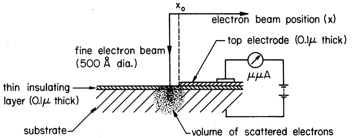
Fig. 1. Schematic view of experimental arrangement.
