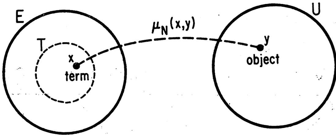
Fig. 1. The components of a fuzzy language:  $U$  = universe of discourse;  $T$  = term set;  $E$  = embedding set for  $T$ ;  $N$  = naming relation from  $E$  to  $U$ ;  $x$  = term;  $y$  = object in  $U$ ;  $\mu_N(x,y)$  = strength of the relation between  $x$  and  $y$ ;  $\mu_T(x)$  = grade of membership of  $x$  in  $T$
