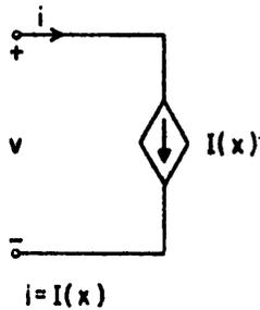
(c) x-controlled linear resistor
