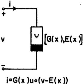
(b) x-controlled convex resistor
